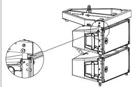
4) Reverse and connect the 1 rear bracket to the fly-bar using 2 quick lock pins. The first HDL has to be fixed always starting at  $0^{\circ}$  with respect of the frame. No other angles are allowded.
