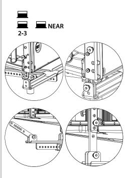
Usually, the cluster switch on the input panel should be set to the 2-3 position and the HF on NEAR when a single speaker is used. Indoor switch use depends on the speaker placement. Place the speaker or the pole on a tripod using its own hardware LIGHT BAR HDL20-A (P.N. 13360229) or LIGHT BAR HDL10-A (P.N. 13360276) as shown in the following picture.
