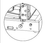
2) The stacking bar adds a fixed amount of up or downtilt to ground-stacked HDL loudspeakers, with additional 15 degrees of adjustment possible (from  $+7,5^{\circ}$  to  $-7,5^{\circ}$ ).
