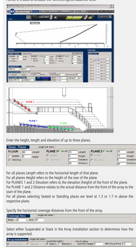
In Suspended mode the grid is suspended and cabinets are attached beneath. In Stack mode the grid forms a base and cabinets are placed on top.
