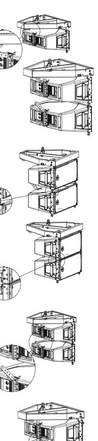
HDL allow users to choose from different face-to-face angle adjustments to create arrays with varying curvature. Thus, designers can create arrays custom-tailored to each venue's profile.
