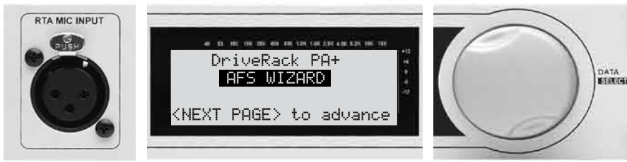
31A - The first screen of the AFS Wizard appears on the display.
