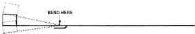
Figure 4-6. RHODES Damper Arm - Alignment Adjustment
