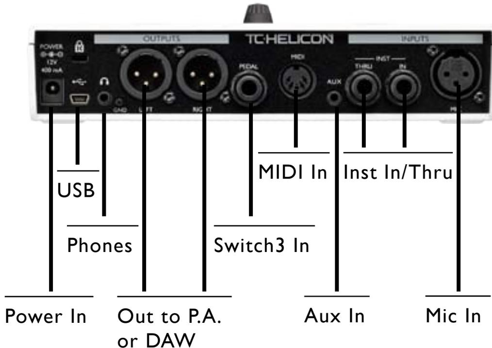
**Power In** - Connect the included power supply (ALWAYS USE A TC-HELICON POWER SUPPLY. USING ANY OTHER POWER SUPPLY MAY DAMAGE THE UNIT AND WILL VOID YOUR WARRANTY.)
