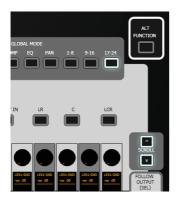
In the GLOBAL MODE section press the BUS 17-24 button and then use the SCROLL arrow buttons to locate LEX1.
