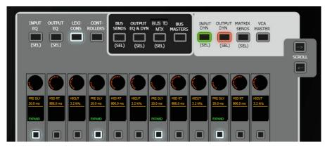
You will now see that there are 4 Lexicon processors assigned to the upper row of encoders. The touch screen will also be showing the menu screen for the 4 Lexicon processors each with the currently active effect preset displayed. Use the ADJUST knob to the right of the touch screen to scroll to the processor you want to edit and then press the Adjust knob to select the processor for editing the FX type.
