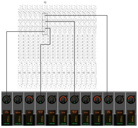
The highlighted controls in the analogue equivalent above represent what will be displayed on the VCS, which is displayed to the right of it, the VCS has been rotated through 90° to make the comparison more complete.
