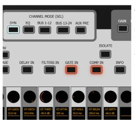
You can now use encoders in the LOWER ROW to adjust the settings for the GATE or COMPRESSOR. You will see GATE and COMPRESSOR activity start to occur on the OLED screen above the input channel you are processing.
