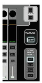
Press the SEL button above the VCA Master fader you wish to assign some input faders too – it will turn WHITE. You may now press the SEL buttons above any of the input channels you want to assign to that VCA Group.
