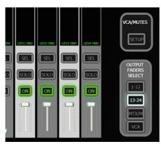
Press the 13-24 button in the OUTPUT FADERS SELECT section.
