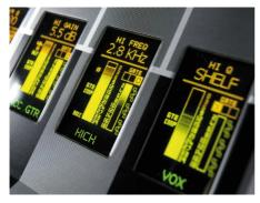
The OLED display is divided into three sections with the top section (the ORANGE part) always describing the function of the encoder situated directly above it.
