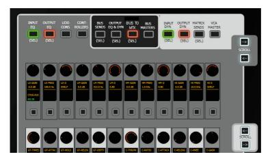
You can now press the SEL button above the Matrix master fader you want to send audio to. The 24 encoders in the central section will be configured as send controls for buses 1-24 to the SEL ected bus.
