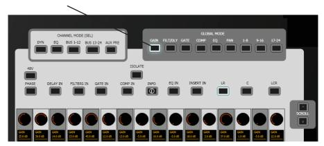
You can now adjust the GAIN control (encoder) just as you would on an analogue console and monitor the amount of input level on the Input Level Meter in the associated OLED display.
