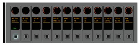
Pressing EXPAND will cause the selected processor to 'expand' across all 12 encoders allowing detailed parameter adjustment. Once you have completed your adjustments, press the CLOSE button to return to the 'compressed' view.
