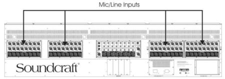
The Mic/Line Inputs on the rear of the console are arranged in 3 or 4 identical blocks with 16 Inputs and 8 Outputs on each giving a total of 64 (48 on Si2, 32 on Si1) Mic inputs. Each block of I/O is labelled either A, B, C or D and these blocks of inputs are mapped to the faders as follows:
