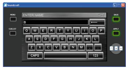
Press the BACK button to exit the naming page and return to the BUS 1 SETUP display.
