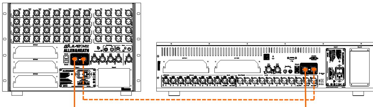
Switch on the MixRack first, then the Surface. The gigaACE Lnk/Err indicators flash at a steady rate when the link is established. The red error indicator lights if a communication error is detected. Check that the cables are correctly plugged in and are not faulty.
