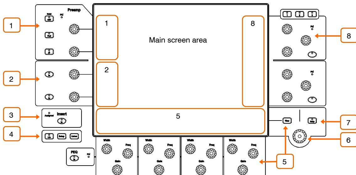
1 **Preamplifier** – Peak indicator and dedicated preamp controls for analogue Gain, Digital Trim, 48V, Pad and polarity.
