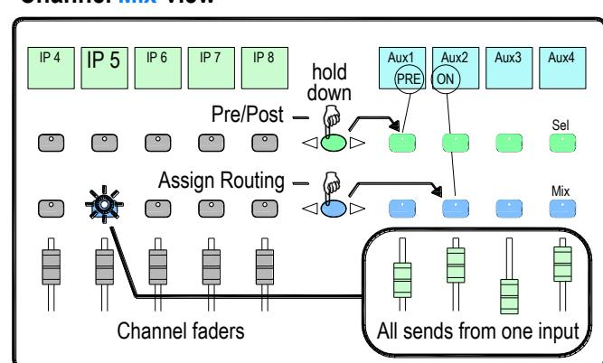
Press an Input Channel strip **Mix** key.
