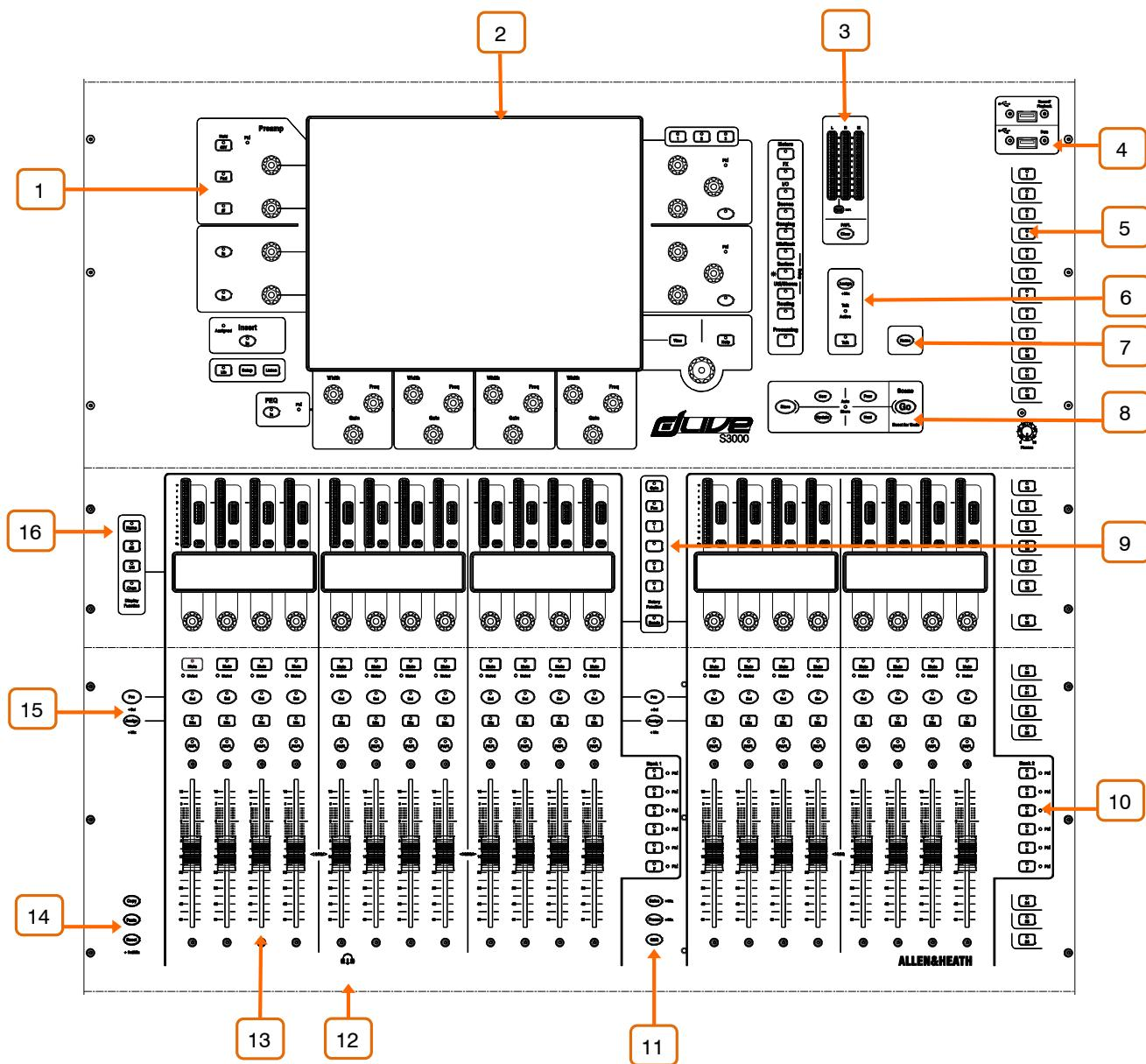
**1 Channel Processing** – Press a fader strip **Sel** key to access the processing for the input or mix channel assigned to it. Read the Harmony UI paragraph below for further information.
