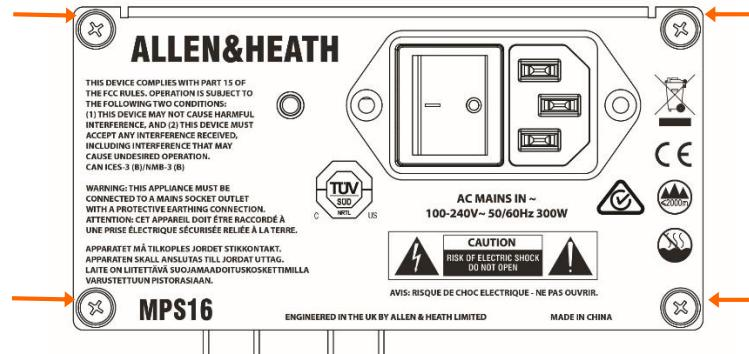
① dLive Surfaces ship with one PSU fitted. A second PSU can be fitted for redundancy (part number MPS-16). Loosen the 4 captive thumb screws securing the blank panel\*, slide the PSU into the slot, and tighten the 4 captive thumb screws indicated above. The Surface will automatically switch between the supplies without interruption to the audio should one fail.
