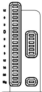
**Meter** – 22-segment signal meter and 6-segment gain reduction meter. The meter displays audio signal activity for the channel.
