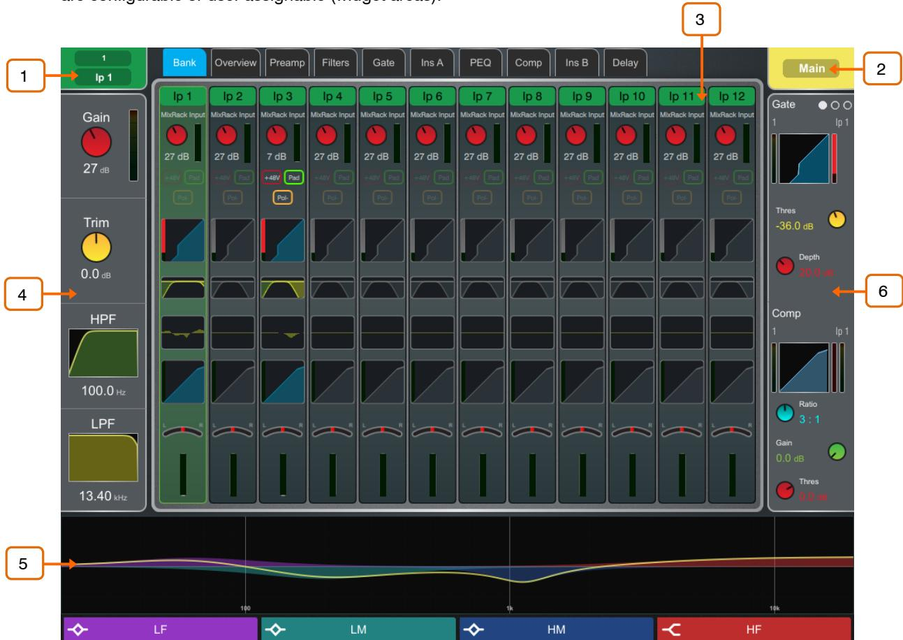
**1 Selected channel** – Displays the name, colour, type and number of the currently selected channel. Tap to edit channel name and colour. 7 colours and off are available.
