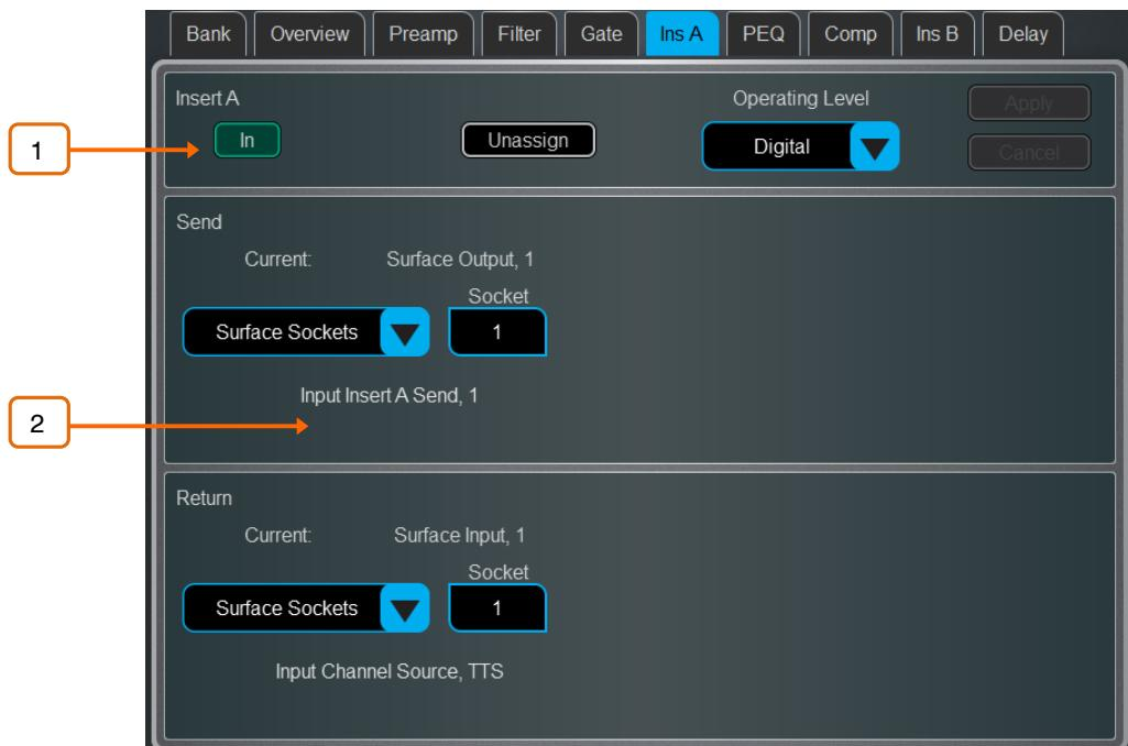
**1 Insert Settings** – Press **In** to switch the inserted device in circuit. Choose the **Operating Level** of the insert point: Digital sends the signal at 0dB for use with external digital equipment via AES3 or I/O Ports; Analogue compensates for the +4dBu nominal level on the XLR outputs, so that the overall gain of the insert circuit is 0dB; -10dBV is a standard for consumer equipment. Press **Unassign** to clear the current Insert assignment.
