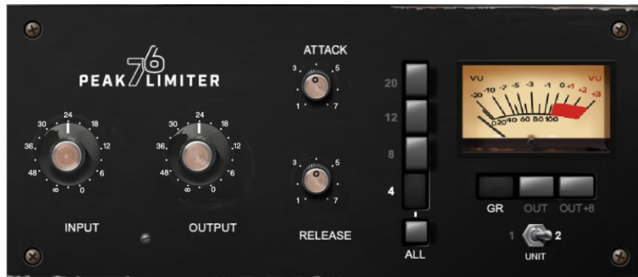
**Peak Limiter 76** - A faithful emulation of the legendary FET limiting amplifier from the late 60s, complete with its nonlinear distortion characteristics, program-dependent Attack, Release and Ratio settings, and trademark 'All buttons' mode.
