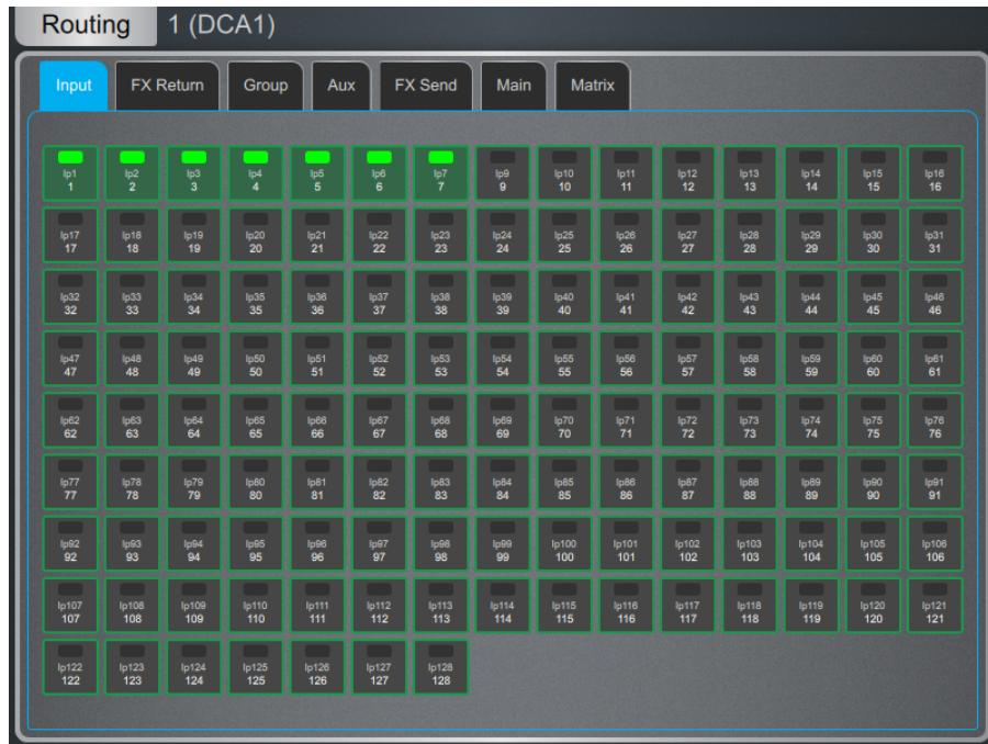
**DCA and Groups** – Displays channel assignments to the DCA or Group. Touch **On/Off** to toggle the channel assignment to the DCA or Group. For DCAs, use the tabs on top to display different channel types.
