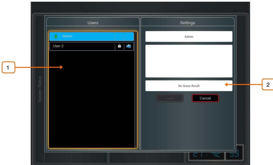
1 **Users list** - Shows available Users. These can be configured and enabled in the **MixRack / Config / User Profiles** screen. The Admin User is always displayed. Icons indicate if the User has a password or User Scene set. Touch a User to select then touch **Login** to change User.
