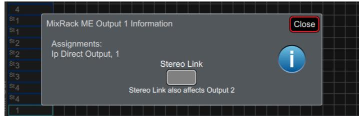
Touch on a ME output to access the Stereo Link option. When Stereo Linked, outputs to the Allen & Heath Personal Monitoring System will be recognised as a stereo pair and assigned to a single key on the ME-1 mixer.
