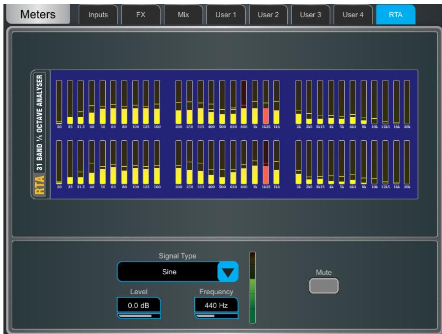
**RTA** – A 1/3 octave Real Time Analyser for the active PAFL signal.
