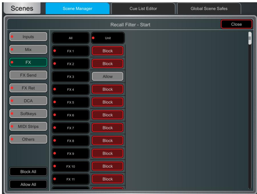
**Recall Filters** – A Recall Filter prevents certain channels or parameters being overwritten by the Scene recall. It only affects the Scene it is associated with.
