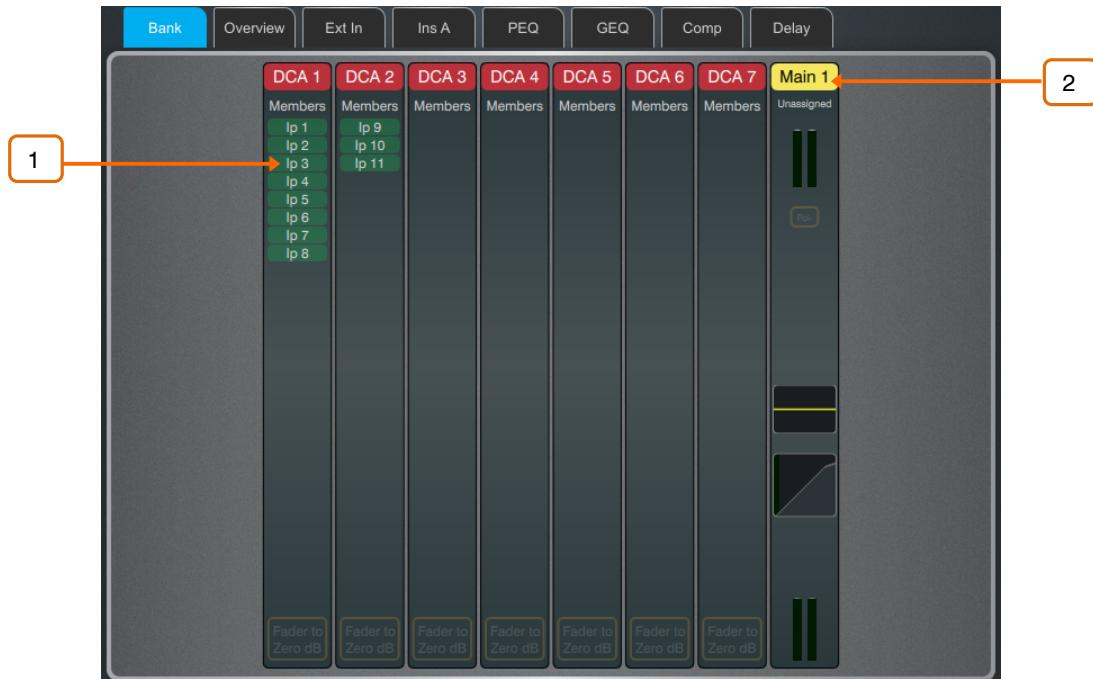
**DCAs** – Displays name, colour, members (assigned channels) and whether the 'Fader to Zero dB' option is enabled. Use the **Routing** screen or the Surface **Assign** keys to assign channels.
