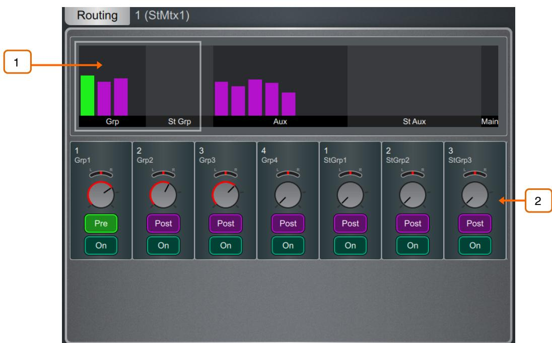
**Matrix sends** – Displays routing and assignments of Groups, Aux and Main mixes to the selected Matrix.
