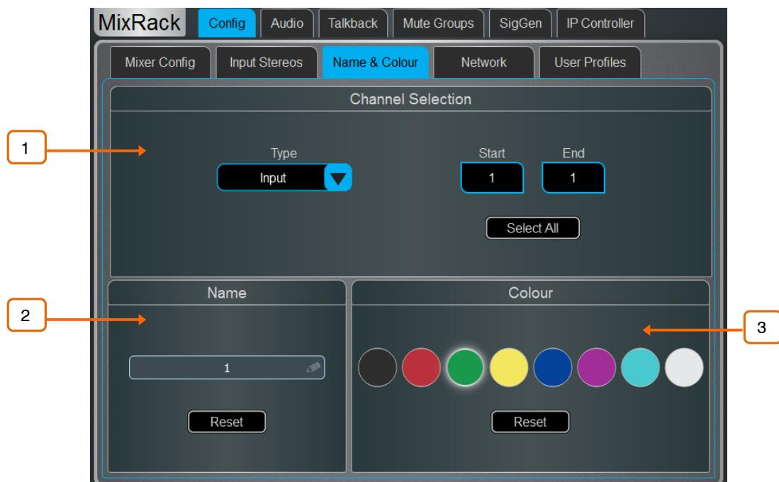
**1 Channel Selection** - Set the channel **Type** from the drop-down menu. Touch **Select All** or set the **Start** and **End** to select a range of channels.
