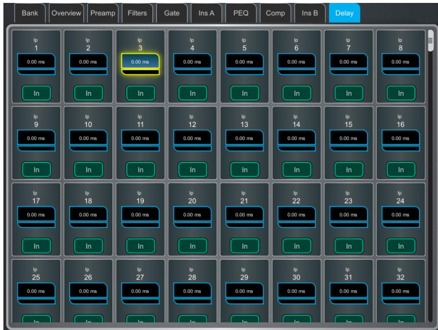
➊ Hold down **Setup** and touch anywhere in the Delay page to access the unit and temperature preferences for the Delay. The default unit is ms but can be changed to metres, feet, or samples. This can be changed globally for the Input channels and for the Mix channels. Enter the ambient temperature if using distances so that dLive can compensate for the effect on delay.
