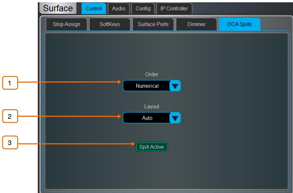
**1 Order** – The order in which the channels are displayed on the Surface. Set to **Numerical** to follow the channel number, or **Strip** to follow the order of the strip layout at the moment of the spill.
