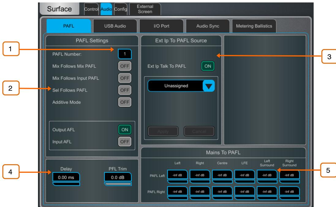
**1 PAFL Number** – Set the PAFL bus that the Surface will use for the monitoring system. This affects the function of the PAFL keys, Listen key, and audio to the Surface headphones.
