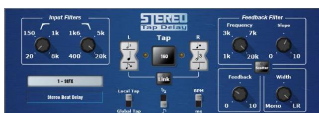
**Stereo Tap Delay** - Provides a clean digital delay with a maximum delay time of 2.7 seconds. One of the key features of the stereo tap delay is the ability to
