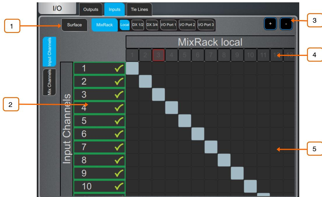
1 **Navigation tabs** – Touch on an item to present its associated sources or channels to the matrix view.
