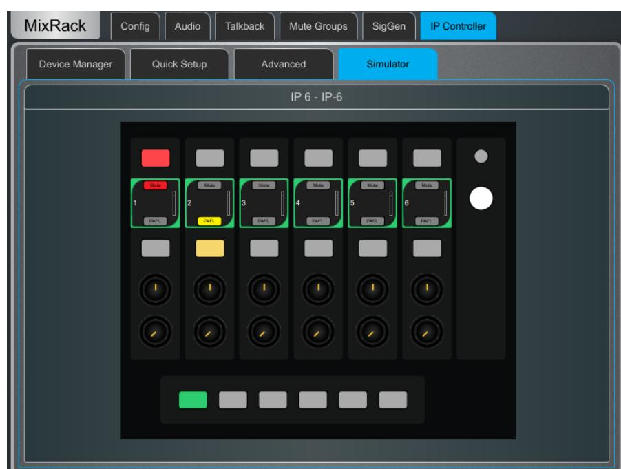
Touch a key on the screen to control the assigned function. Touch a fader / rotary control and use the Surface screen rotary encoder to control the assigned parameter.
