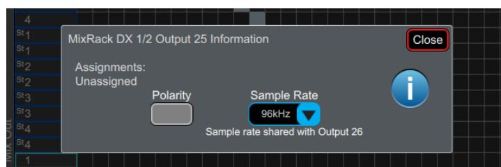
For example, touch on a DX32 digital output to access its Polarity and Sample Rate settings.
