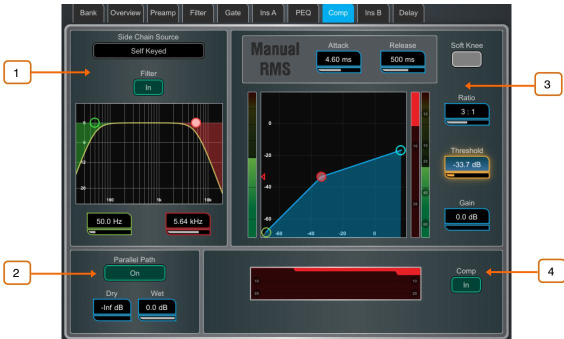
**1 Side Chain** – Touch the **Side Chain Source** box to open a window for selecting the Key (trigger) input to the Gate. An adjustable HPF and LPF filter can be switched in to limit the frequency range of the Key signal. The curve turns yellow when the filter is switched in.
