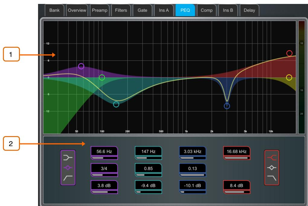
1 **Graph** – Touch and drag the 4 band dots to adjust their centre frequencies. Touch and drag the HPF / LPF dots to adjust their cut-off frequencies. The overall frequency response curve turns yellow when the PEQ is switched in and grey when switched out.
