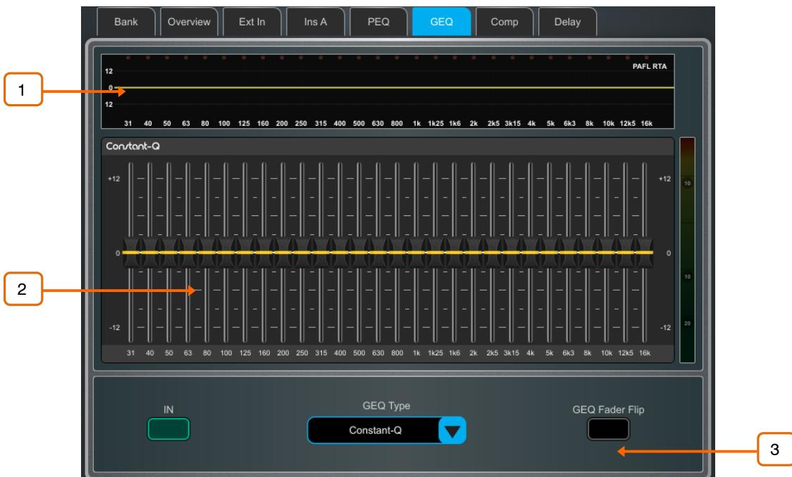
**1** **Graph** – The top part of the screen shows the combined frequency response curve of the GEQ. The curve turns yellow when the GEQ is switched in and grey when switched out. An RTA of the PAFL signal with optional peak band indication is also superimposed on the graph.
