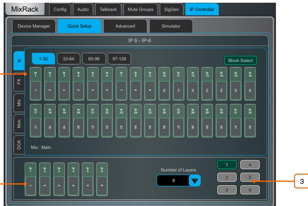
✿ Before you start, hold down **Setup** and touch anywhere in this screen to edit the default settings for Quick Setup. These settings determine the function of the strips at the moment of assigning to the IP device. They don't affect strips which are already assigned.
