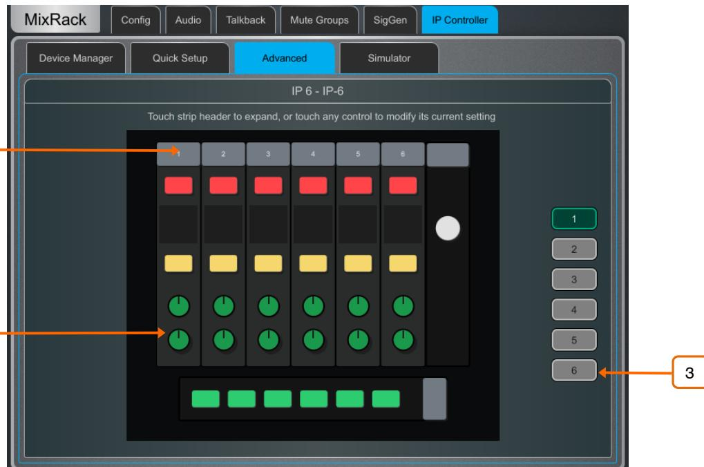
1 Touch a strip header to expand the view and display the assigned functions or parameters for the strip.
