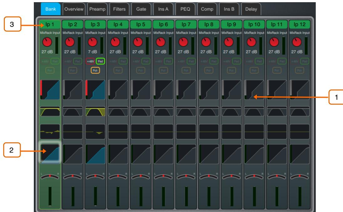
**Input channels** – Displays name and colour, source type, preamp meter, gain, +48V and polarity, gate graph, filters, PEQ graph, compressor graph, Pan and channel meter. The channel name is framed in orange when Virtual Soundcheck is active.
