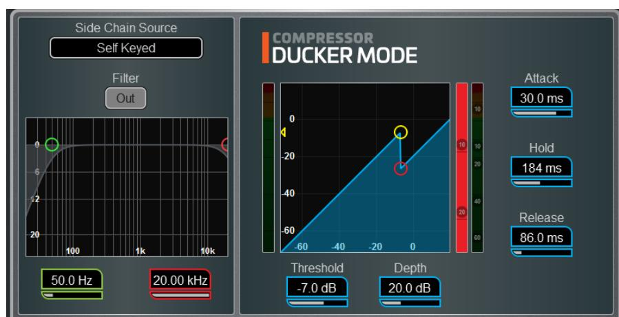
**Ducker** - The Library for the Gate and Compressor processing blocks includes a channel Ducker with key source selection and LPF/HPF filters, plus controls of Threshold, Depth, Attack, Hold and Release.
