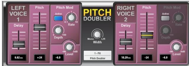
**Pitch Doubler** - PitchDoubler is a stereo, pitch shifting doubler effect generating the effect of additional voices from its input. It is based on the same pitch shifting technology as VocalShift, with the associated low latency (<6ms), wide frequency range (down to around 80Hz) and minimal phasing / flutter artefacts. The effect squeezes two channels of high quality pitch shifting into a single effect slot, along with further features such as adjustable delay and modulation.
