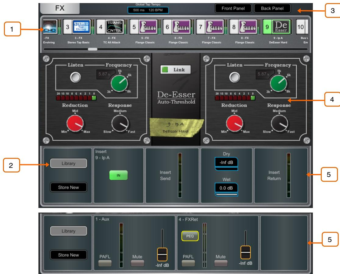
**1 FX bar** – The 16 slots are shown across the top of the screen either empty or with FX devices loaded. The FX name, current Library preset and metering is shown next to each icon. Scroll left to right to view all the FX slots. Touch a device or empty slot to select.
