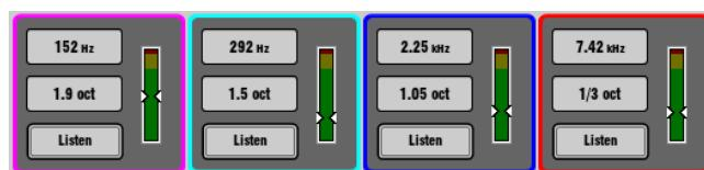
**Frequency control** - All 4 bands are full range 40Hz - 18kHz.
