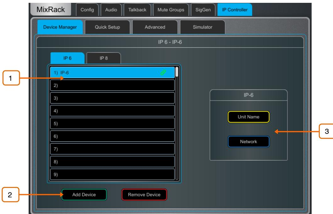
**1** Select the device tab using the tabs on top, and select one of the 16 locations in the list. The list shows the unit name of assigned devices.
