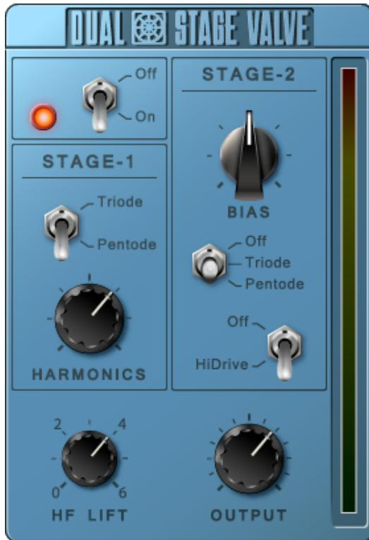
**Dual-Stage Valve** – Inspired by a known studio preamplifier, this model recreates the distortion characteristics of valve circuits, from very subtle coloration to full overdrive. It can be fully bypassed with the **On/Off** switch.
