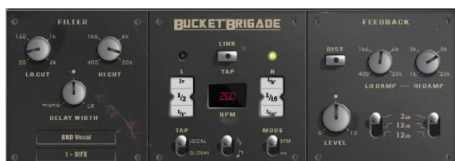
**Bucket Brigade Delay** - This is an emulation of a vintage analogue delay unit that used a 'bucket brigade device' (BBD) chip for the delay. This was a discrete analogue time delay line where the stored analogue signal was moved along a series
