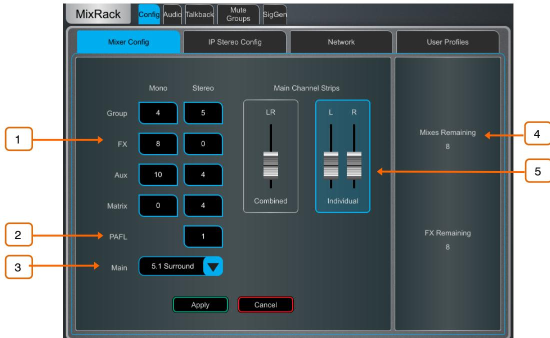
**1 Bus configuration** – Touch a box and use the screen rotary to set the number of mono / stereo Groups, FX sends, Aux sends and Matrix outputs. You can choose any combination, but note that mono busses can only be added / removed in pairs.
