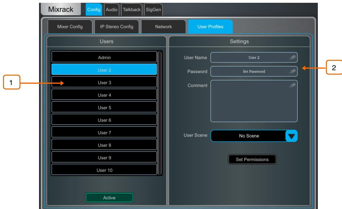
**1 Users** – The Admin user has access to all functions and can set permissions and allocate passwords if required for the other users. The password, if one is set, is required when the User logs in, changes User or locks / unlocks the dLive Surface. Icons in the list indicate if a password is set and if the User is active.
