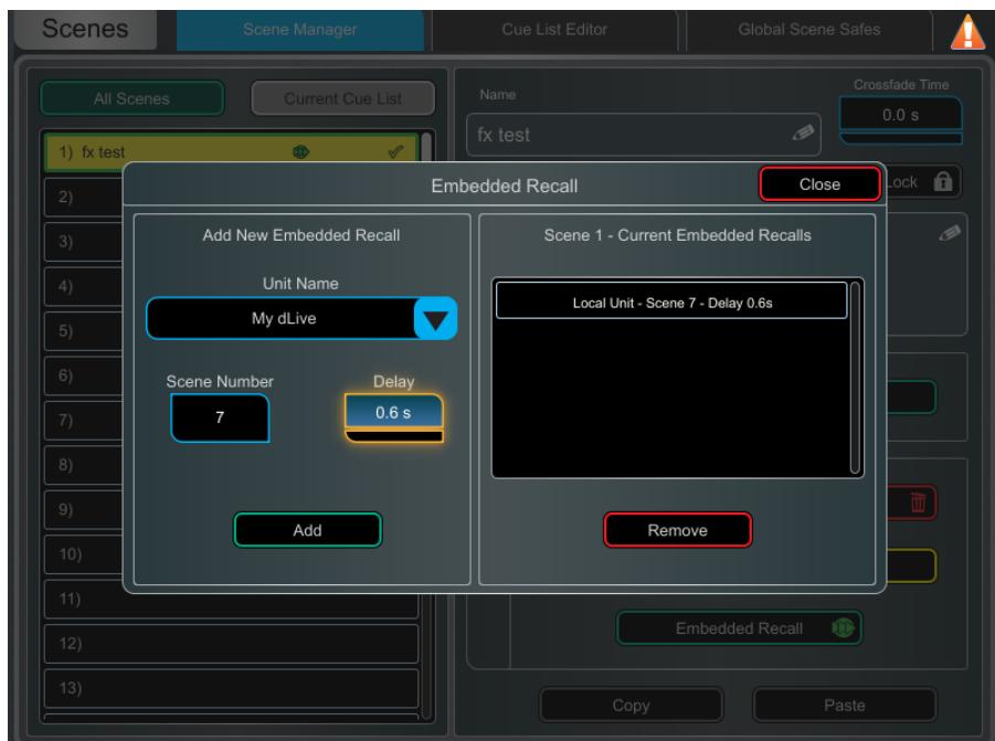
**Embedded Recall** – You can automate the recall of one or more other Scenes from the same or a different unit when you recall a Scene. A delay time can be set for each embedded Scene within the host Scene.
