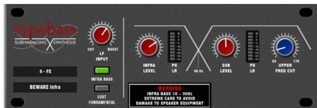
**Hypabass** - A sub-harmonic synthesis unit used in the live sound environment to generate infra and sub bass spectrum from weaker bass programme. We initially emulated the American analog classic, but implementation in DSP gave us the ability to use more sophisticated techniques in the sub harmonic generator and filtering
