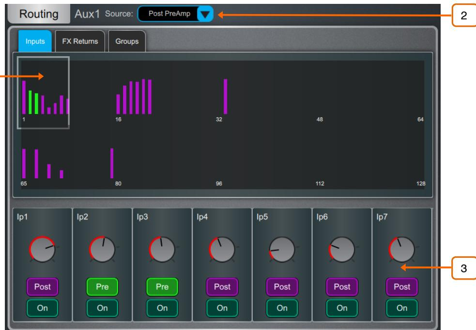
**Aux and FX sends** – Displays routing and assignments of Input channels, FX Returns and Groups to the selected Mix.
