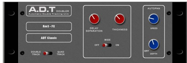
**ADT Doubler** - An Automatic Double Tracking module capable of creating short echo/chorusing, classic double tracking and 'slapback' tape delay loops.
