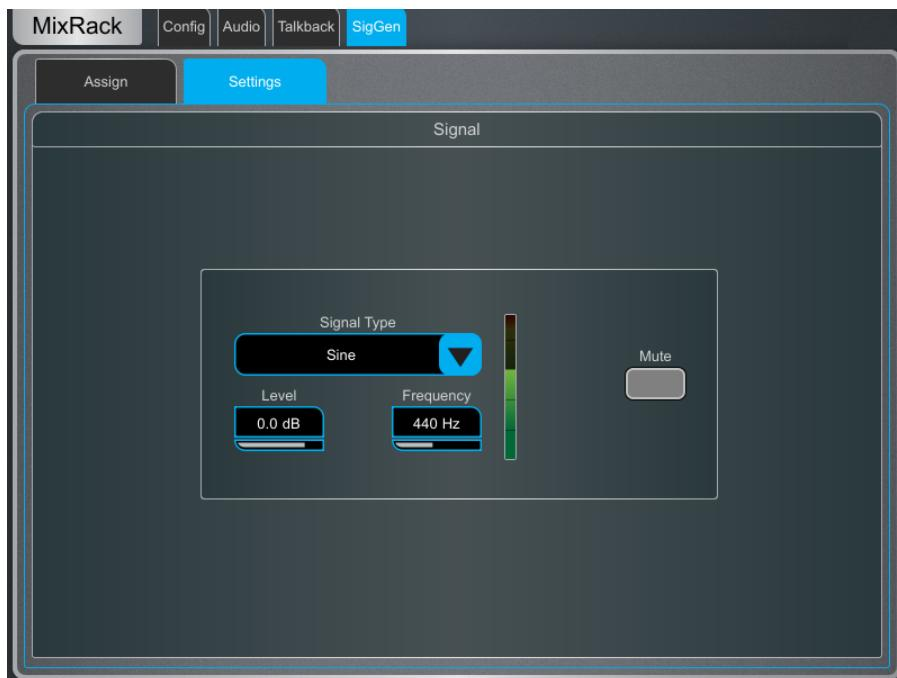
**Settings** – The SigGen **Level** can be set from fully off to full scale +18dB. Touch the **Mute** button to turn off.
