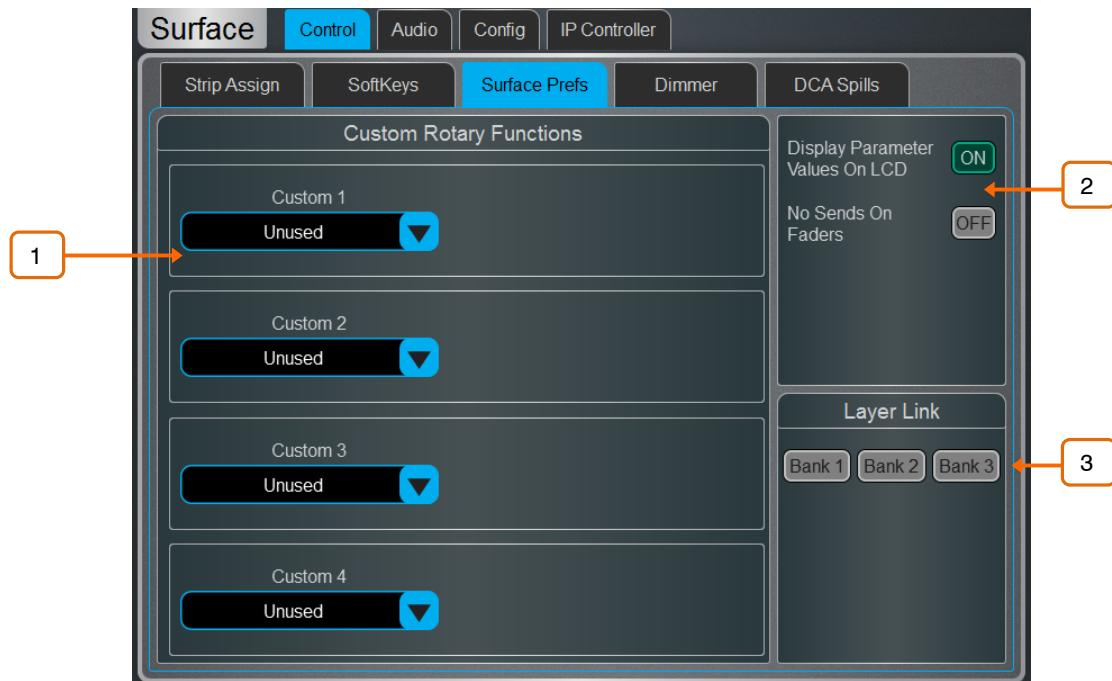
**1 Custom Rotary Functions** – Use the drop-down menus to select the required **Function** for each Custom strip rotary control. Available functions are Unused, Direct Out, Send Level (Aux or FX sends), HPF Frequency, Compressor Threshold, and Channel Level. Touch **Apply** to confirm the change.
