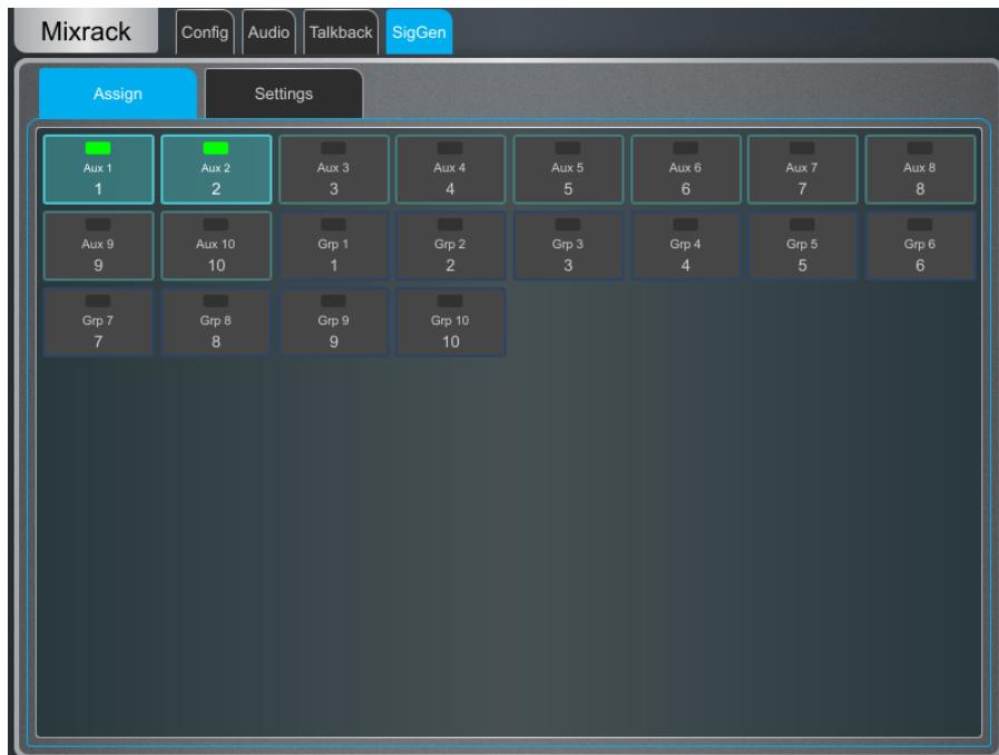
**Assign** – Touch a Mix button to assign the SigGen. The signal routes through the Mix processing, therefore will be affected by the Mix EQ and compressor.
