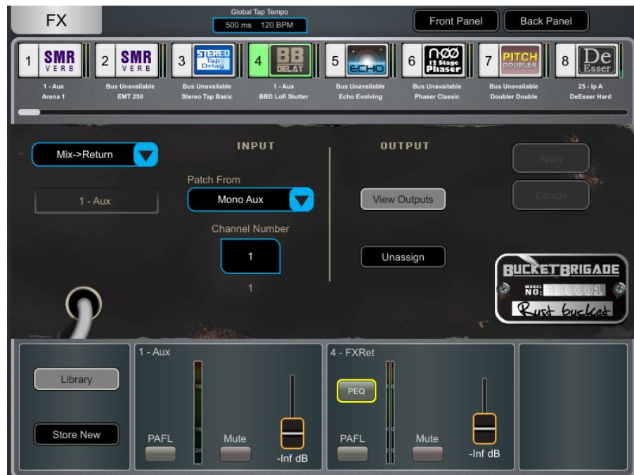
**Back Panel** – Use this view to edit the routing for the selected FX. Use the drop-down box to choose between Unassigned, Insert or Mix->Return.
