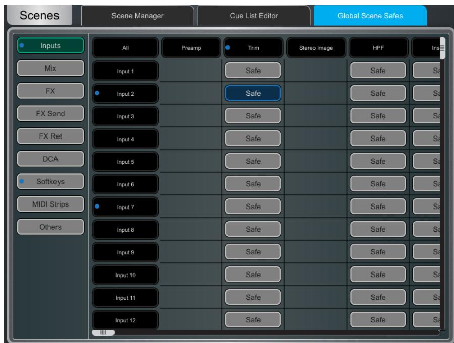
Use the tabs on the left to view the different parameter groups. Swipe up/down or left/right to navigate through the table. Touch an item to toggle its state. Safe items (highlighted in blue) will not be recalled.
