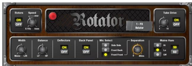
**Rotator** - The Rotator is a model of a traditional rotary speaker cabinet such as those used to create the familiar Leslie organ sound. It simulates the rotating horn (treble) and woofer (bass) along with their crossovers.
