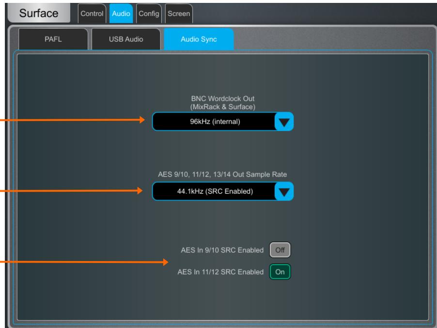
**1 BNC Wordclock Out** – Select the sample rate for the Wordclock output provided at the Surface and MixRack. This can be set to **Off**, **44.1kHz**, **48kHz** or **96kHz (internal)**.
