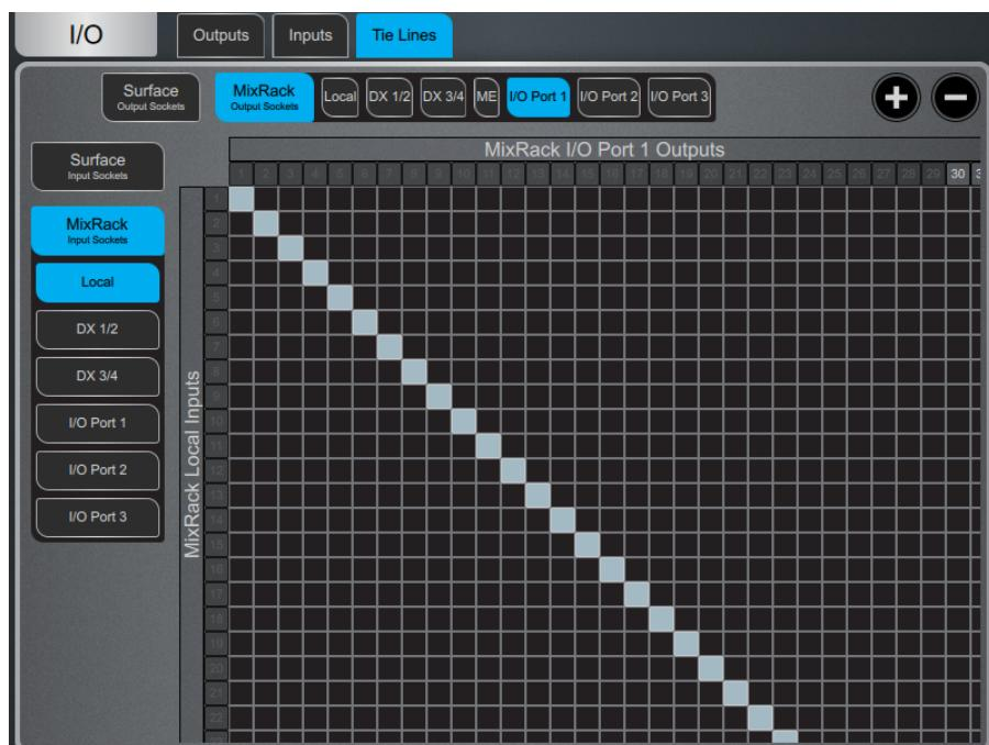
**Digital Split using Tie Lines** – In a digital split system (for example FoH and Monitors), it is typical to use the Tie Lines to send the Local inputs from the Master MixRack to an I/O Port and over to the Slave system, as pictured above. This method (as opposed to using channel Direct Outs) splits the signals straight after the preamp so they are unaffected by Digital Trim or Direct Out Source on the Master system.
