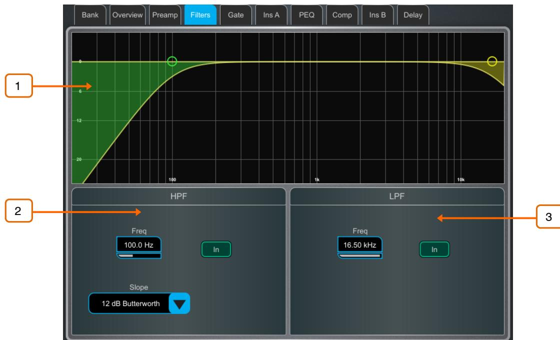
**1 Graph** – Touch and drag the HPF (green) or LPF (yellow) dots to adjust the filter cut-off frequency.
