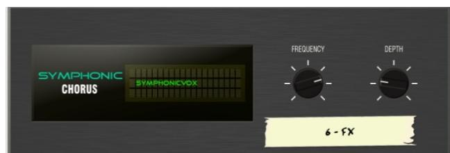
**Symphonic Chorus** - A faithful emulation of the 80's classic chorus effect. Simple to use and frequently requested. The unit has just two controls, Frequency and Depth, controlling the rate and delay range of the stereo modulator. The unit produces a rich, lively and wide chorus sound with a suggestion of very mild phasing / flanging.
