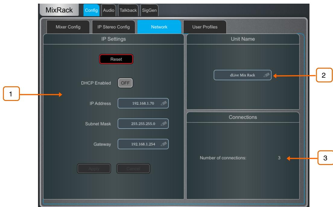
**1 IP Settings** – To set a static IP Address, touch the **IP Address** box and type in the address. Make sure the Subnet Mask and Gateway are valid, and all devices on the network including Wi-Fi routers, access points or laptops have unique but compatible addresses.
