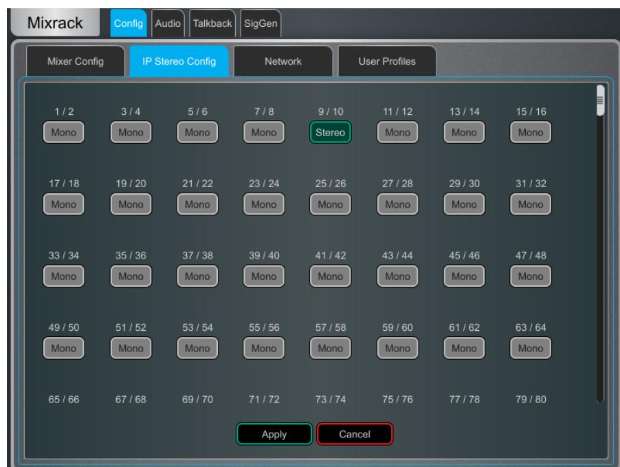
**i** This is intended for permanently configuring channels as stereo inputs, for example music players. Use the **Ganging** screen for on-the-fly linking of stereo sources while mixing live.
