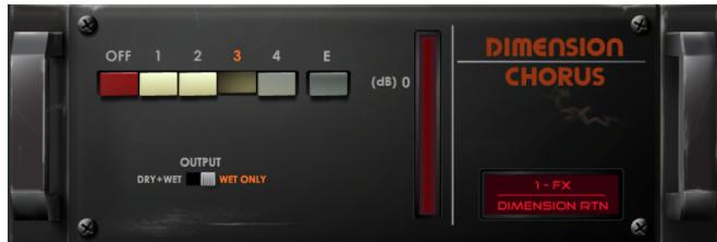
**Dimension Chorus** – A model of a classic chorus device based on bucket-brigade technology. The 4 modes offer varying degrees of density from subtle spatial chorus to heavy modulation, with mode 'E' extending beyond the capabilities of the original outboard unit.
