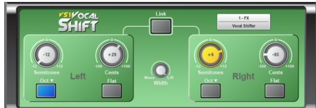
**VS1 Vocal Shift** - VocalShift VS1 is a stereo vocal pitch shifter squeezing two channels of high quality pitch shifting into a single effect. It has a very low latency (<6ms), covers the whole vocal frequency range, and minimises the phasing and flutter artefacts common with many pitch shifters.
