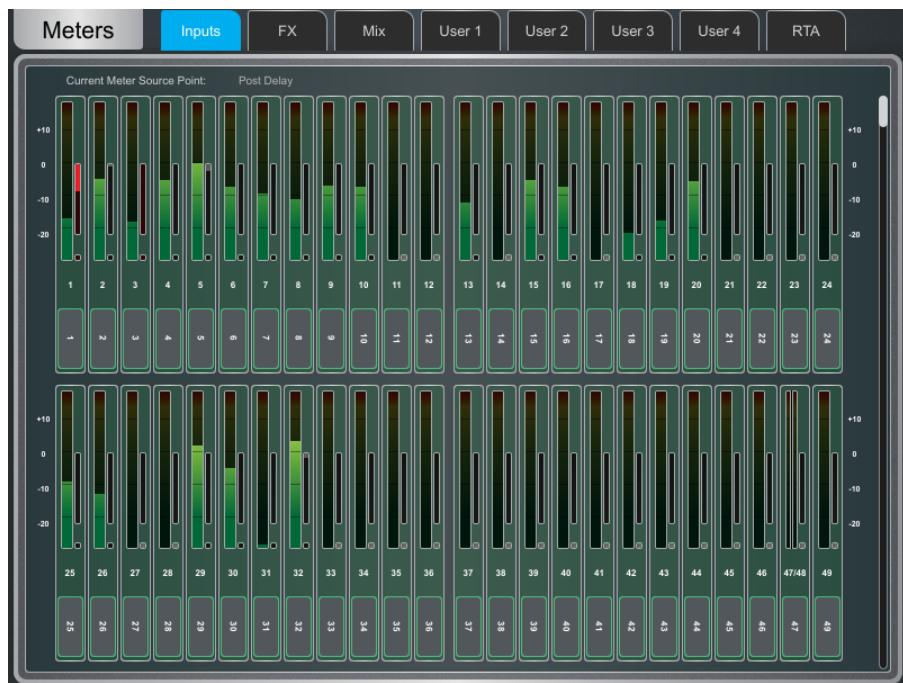
**Meters tabs** – Channel name and colour is shown below each meter. A gain reduction meter and gate active indicator are also displayed, these show activity in red when switched In, and in grey when switched out.
