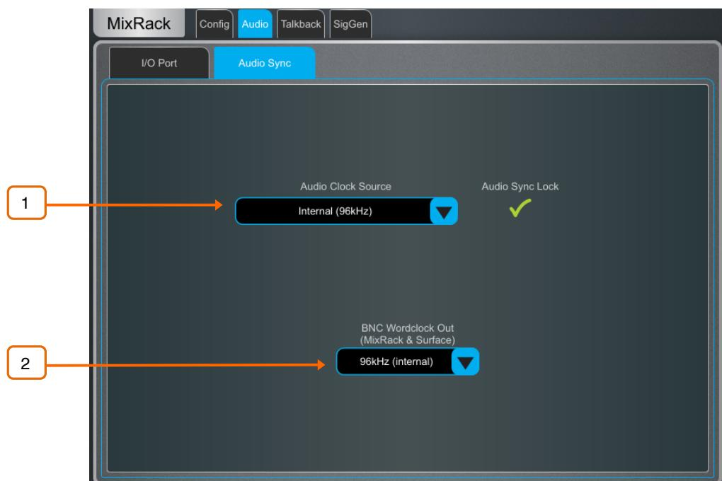
1 **Audio Clock Source** – Select the clock source for the dLive system. Set to **Internal (96kHz)** to use the internal audio clock, this is the default setting. Set to an **I/O Port** to sync from an audio networking card, or **MixRack / Surface BNC Wordclock In** to sync from a 96kHz Wordclock provided at the BNC input of the MixRack or Surface.
