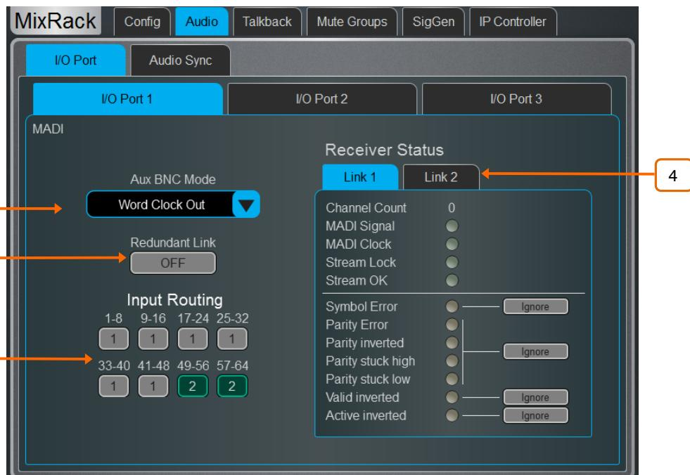
**1 MADI Aux BNC Mode** – Set to **In 1 Thru** to replicate the incoming Link 1 stream to the Aux BNC. Set to **Out 1 Mirror** to split MADI outputs to the Aux BNC. Set to **Wordclock Out** to provide a Wordclock signal on the Aux BNC.
