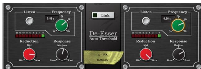
**De-Esser** - Based on the flagship iLive FX engine, the De-Esser emulates the classic Auto-Threshold circuit commonly found on high end hardware units. This produces a constant sibilance reduction regardless of signal level, resulting in a more natural De-Essing process. In comparison, threshold based De-Essing produces inconsistent reduction activity which can result in unnatural vocals.
