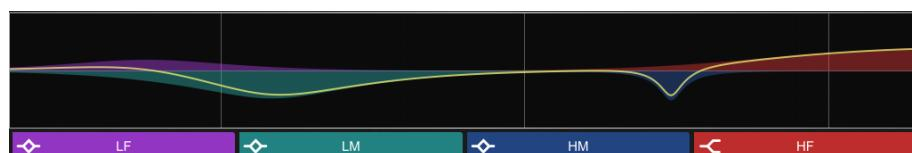
**PEQ Values Only** – Displays value bars for Gain, Width and Frequency.
