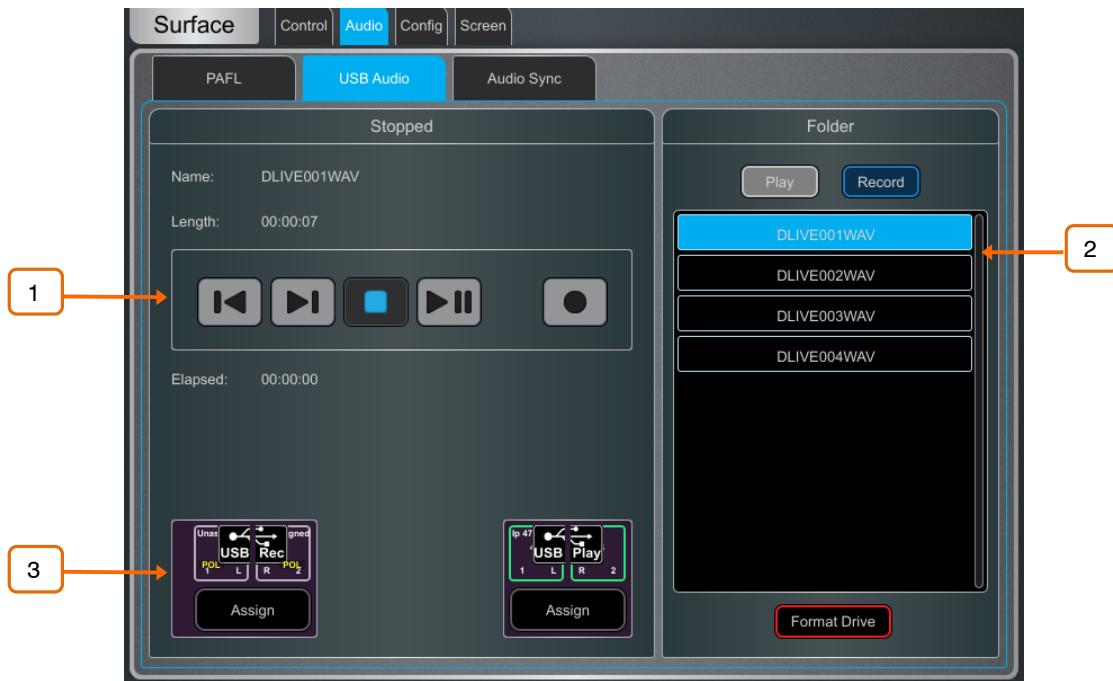
**1** Use the transport buttons to Play, Pause, Stop, Record and select previous or next track. To record, press Record to arm the recording, then press Play.
