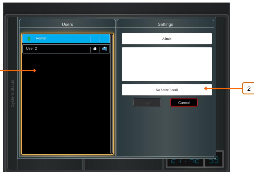
**① Users list** - Shows available Users. These can be configured and enabled in the **MixRack / Config / User Profiles** screen. The Admin User is always displayed. Icons indicate if the User has a password or User Scene set. Touch a User to select then touch **Login** to change User.
