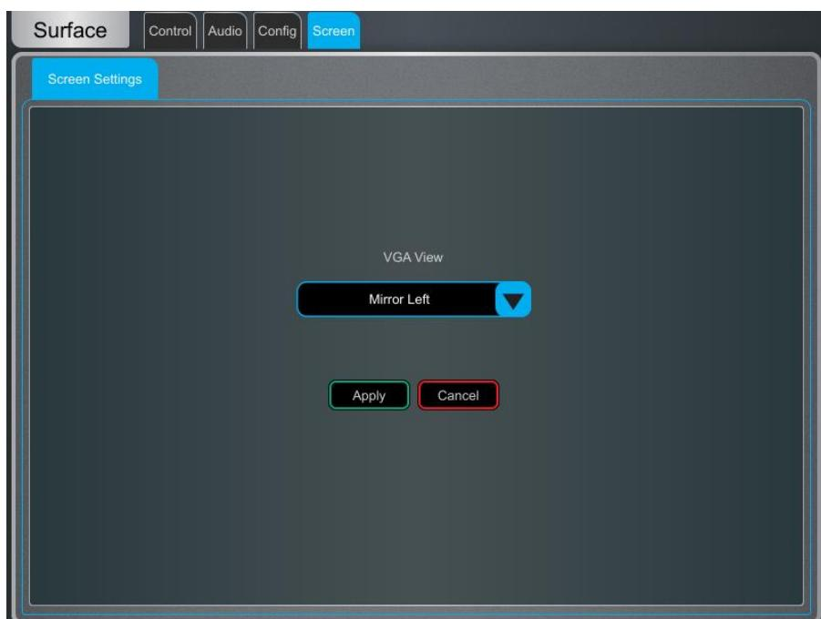
**Screen** – On an S5000 and S7000 you can set the Surface VGA output to mirror either the Processing (Left) or System (Right) screen. The S3000 will always mirror the single screen. Press **Apply** to confirm a change.
