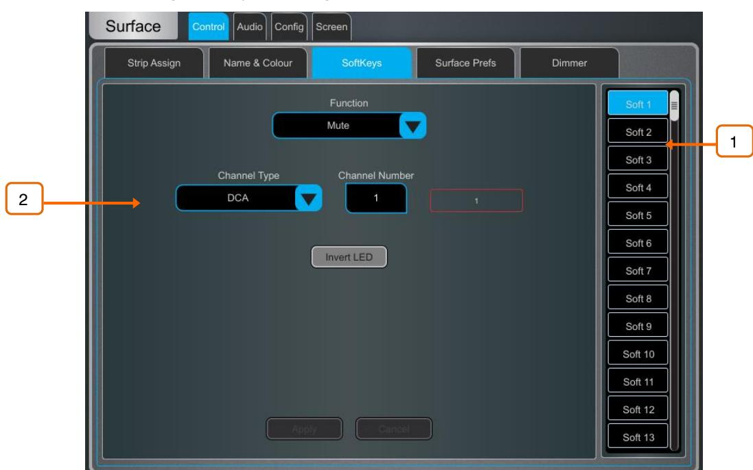
1 Touch one of the SoftKeys buttons on the right of the screen to select it. Swipe up / down to scroll.
