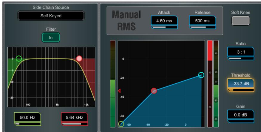
**Manual RMS** - Offers the response of a fairly fast pre-threshold RMS detector with added ability to manually modify the post threshold ballistics for classic sounding RMS compression with additional attack or release smoothing.
