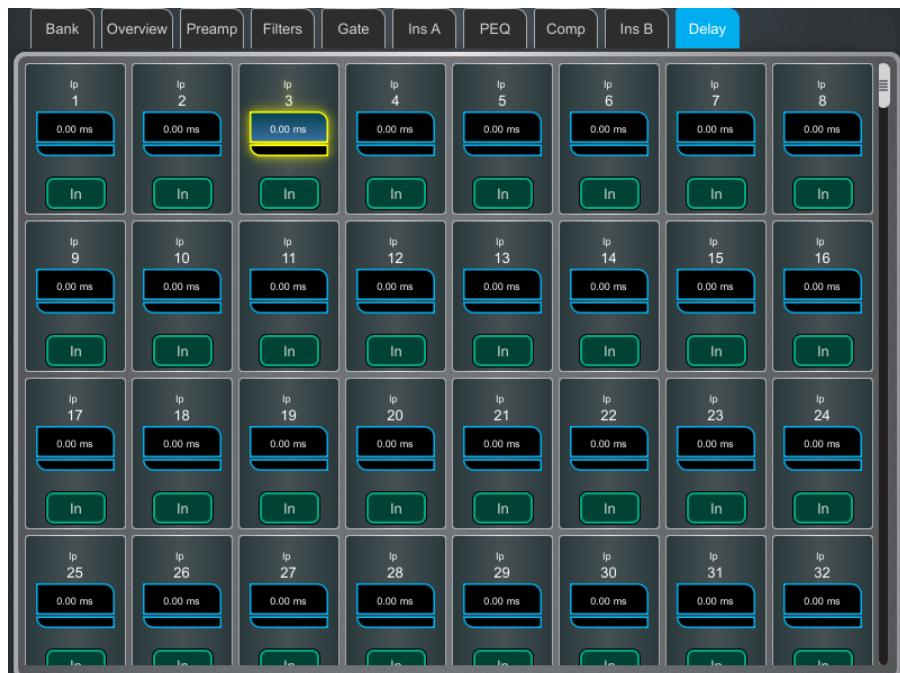
ⓘ Hold down **Setup** and touch anywhere in the Delay page to access the unit and temperature preferences for the Delay. The default unit is ms but can be changed to metres, feet, or samples. This can be changed globally for the Input channels and for the Mix channels. Enter the ambient temperature if using distances so that dLive can compensate for the effect on delay.
