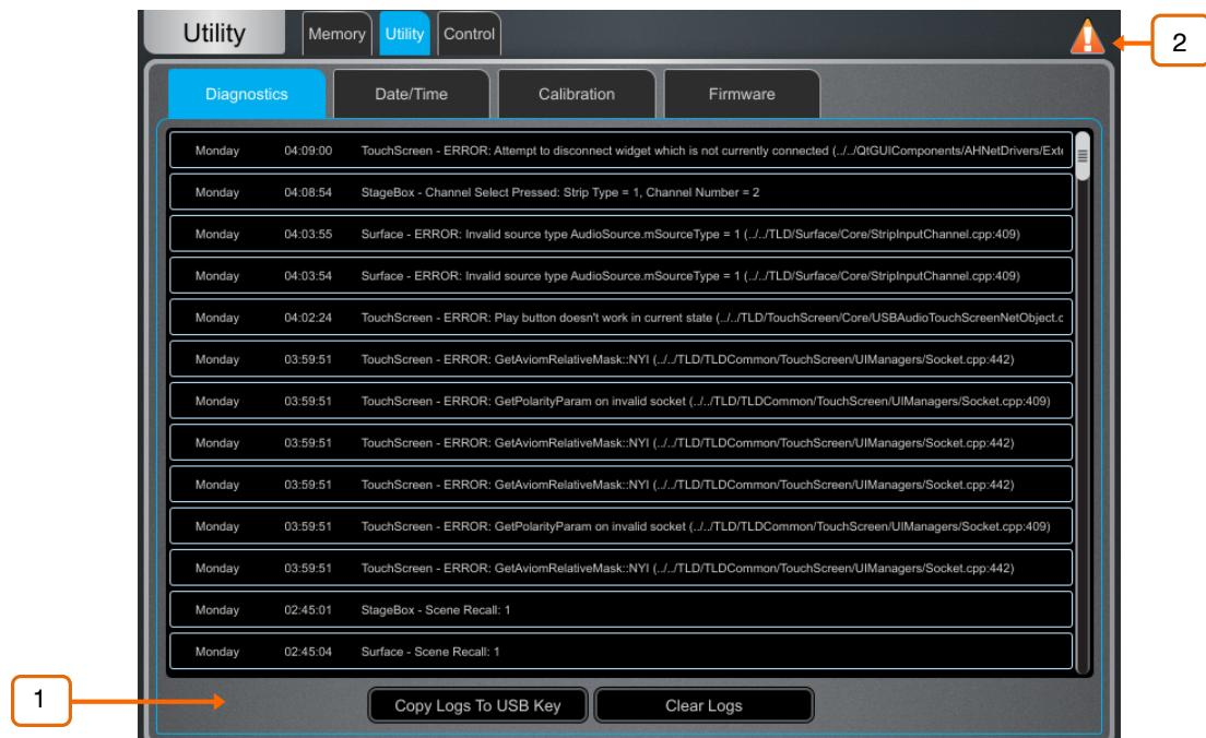
1 If you suspect a problem with the dLive system you can **Copy the logs to USB Key** and send them to Allen & Heath Product Support for diagnostic purposes
