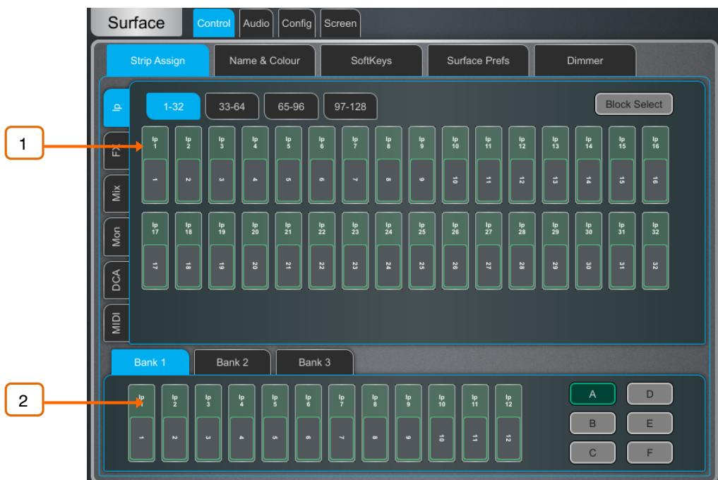
1 Drag and drop channels into the desired position in the lower window. Use the tabs on the left to view different types of channels available, and the tabs on top to navigate to higher / lower number channels.
