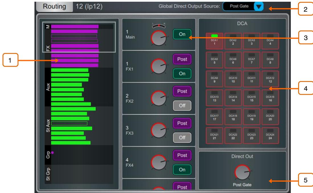
**Input channels** – Displays routing, assignments and Direct Out controls.
