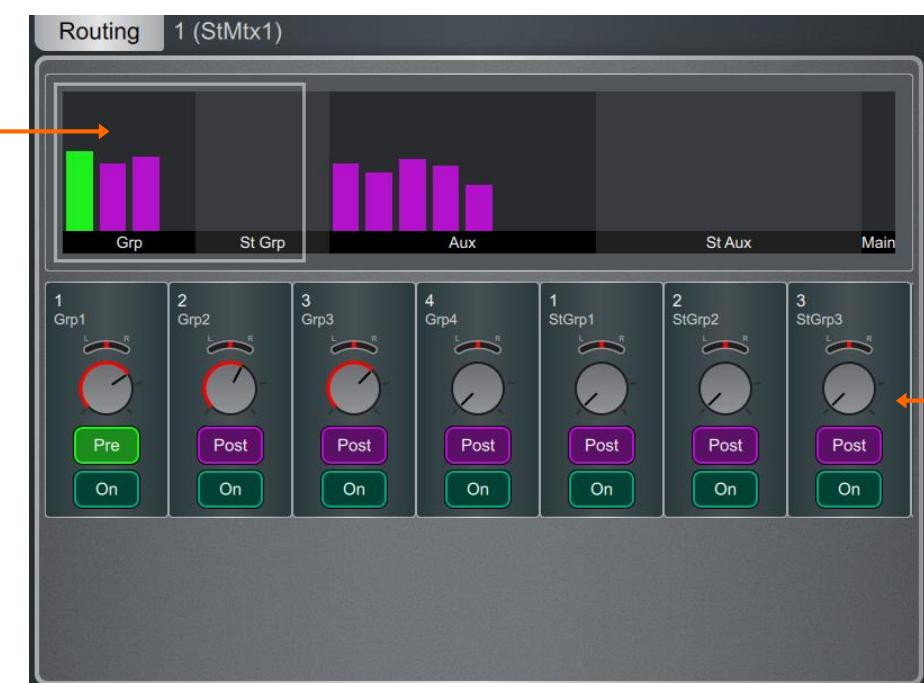
**Matrix sends** – Displays routing and assignments of Groups, Aux and Main mixes to the selected Matrix.
