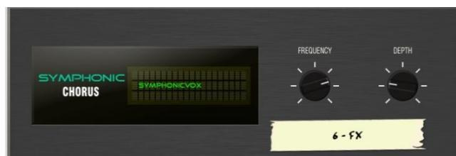
**Symphonic Chorus** - A faithful emulation of the 80's classic chorus effect. Simple to use and frequently requested. The unit has just two controls, Frequency and Depth, controlling the rate and delay range of the stereo modulator. The unit produces a rich, lively and wide chorus sound with a suggestion of very mild phasing / flanging.
