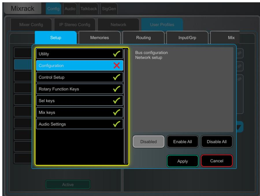
**User permissions** – Each User can have their own set of Permissions applied. Use the tabs across the top of the window to view and set different groups of permissions. Select an item in the list and toggle the **Enabled/Disabled** button as required. The window on the right provides a description of the functions included in the currently selected item. Use the **Enable All / Disable All** buttons to quickly toggle all items in the currently open tab. Touch **Apply** to accept the changes.
