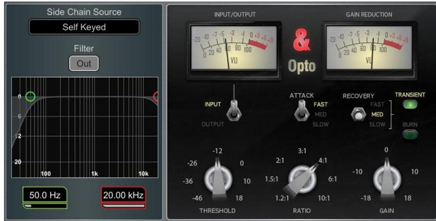
**Opto** - Offers the response of a filament optical compressor. The release has non-linear exponential recovery, fast at the start and smooth for final recovery stage. This creates a smooth and musical sounding compressor.
