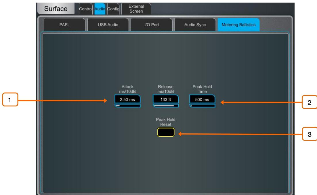
1 Use fast **Attack** and **Release** for fast response, digital absolute peak meters. This ensures you keep control and avoid digital clipping of signals including those with very fast dynamics, but note that the meters may read hotter than those on other consoles you are used to.
