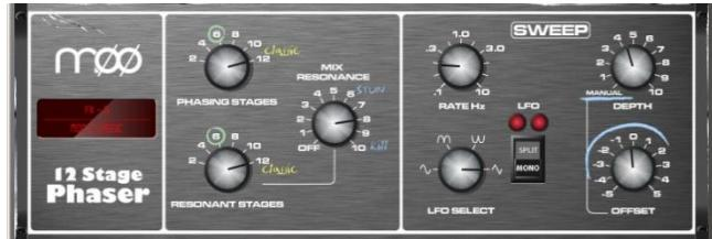
**MOO 12 Stage Phaser** - A classic 12 stage emulation producing rich textured phasing with plenty of control. The user has control of number of stages, feed forward and feed back, and 'zero' depth manual mode – to manually sweep the Phaser using the offset control.
