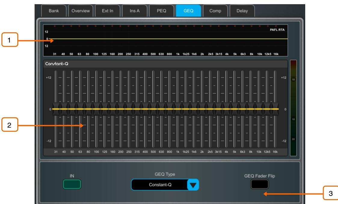
1 Graph – The top part of the screen shows the combined frequency response curve of the GEQ. The curve turns yellow when the GEQ is switched in and grey when switched out.
