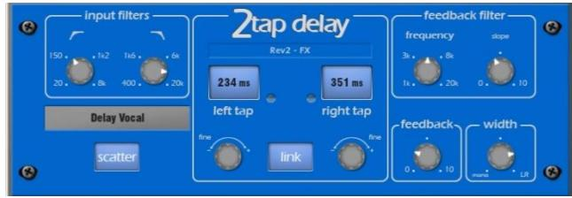
**2-Tap Delay** - Separate left and right tap delay outputs from a mono'd input. Left and right delay can be dialled in using the screen Rotary, tapped on screen or tapped using a SoftKey. Individual tap indicators flash at the tap rate.
