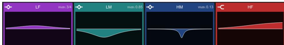
**Multiband PEQ Graph** – Full range PEQ view. The individual effect of each band is shown as fill colours, while the overall response curve is shown as a yellow line. Frequency and gain values are temporarily shown when a setting is adjusted.
