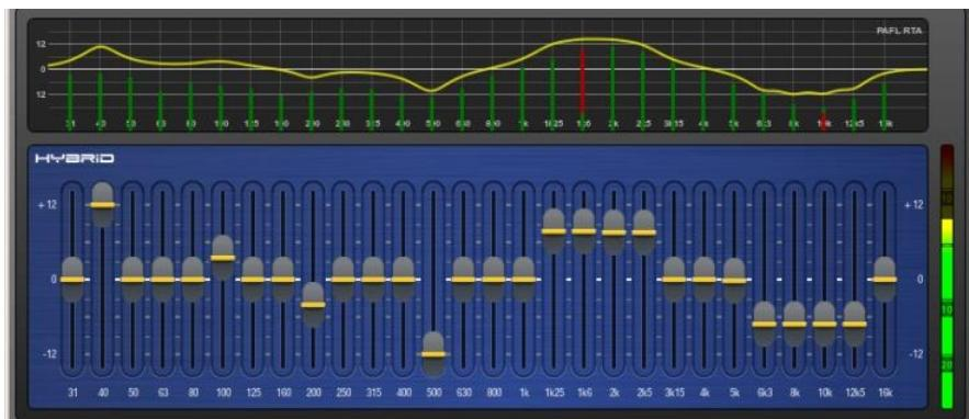
**Hybrid** - Allen & Heath have developed the best of both worlds. The boost is proportional-Q for smooth and warm small boost settings. The cut is Constant-Q providing clinical 1/3rd Octave attenuation with minimal band interaction.
