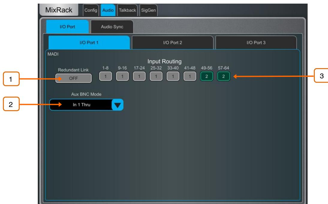
**1 MADI Redundant Link** – Enable this option to use Link 2 on the MADI card as a dual redundant connection.
