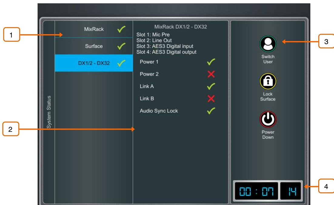
1 **System Status** – Displays a list of system components. A green tick indicates the component is running correctly. A red cross indicates that an error is detected. Touch the component to display further information.
