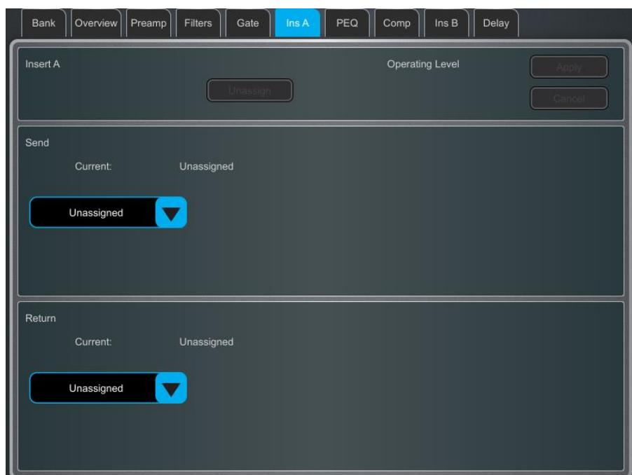
**Insert Unassigned** – Use the drop-down menus to assign the **Send** and **Return** to physical sockets, the I/O Ports or an FX unit. Touch **Apply** to confirm.
