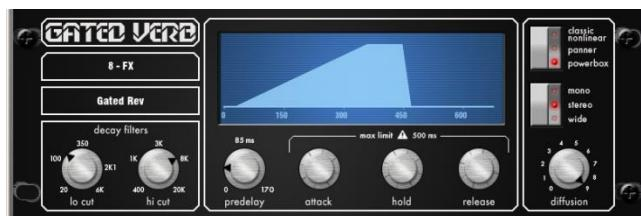
**Gated Verb** - An accurate emulation of the classic 80's Gated Reverb plus two other variants called 'Panned' and 'Powerbox'. The user interface gives instant access to Lo-cut Hi-cut decay spectrum filters and the gate envelope controls - predelay, attack, hold and release.
