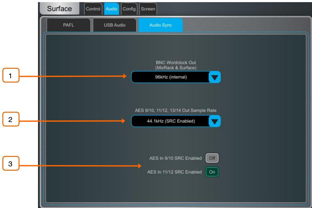
**1 BNC Wordclock Out** – Select the sample rate for the Wordclock output provided at the Surface and MixRack. This can be set to **Off**, **44.1kHz**, **48kHz** or **96kHz (internal)**.
