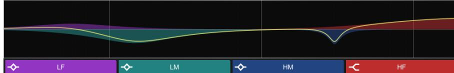
**PEQ Values Only** – Displays value bars for Gain, Width and Frequency.
