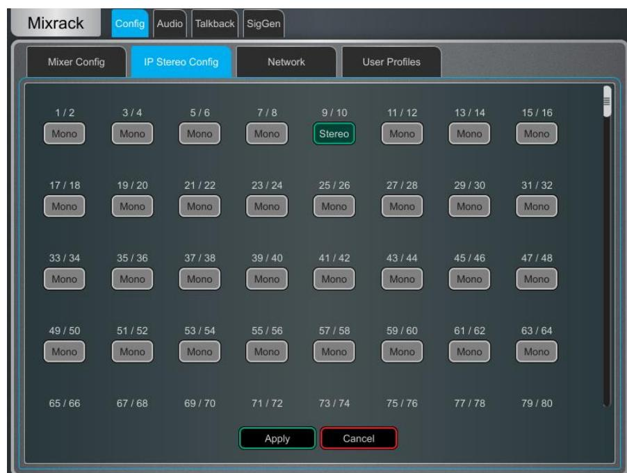
**ⓘ** This is intended for permanently configuring channels as stereo inputs, for example music players. Use the **Ganging** screen for on-the-fly linking of stereo sources while mixing live.
