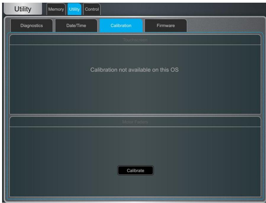
Touch the **Calibrate** button and follow the on-screen instructions, moving the faders to the positions instructed at each step.
