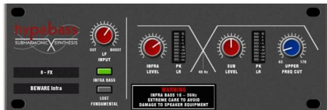
**Hypabass** - A sub-harmonic synthesis unit used in the live sound environment to generate infra and sub bass spectrum from weaker bass programme. We initially emulated the American analog classic, but implementation in DSP gave us the ability to use more sophisticated techniques in the sub harmonic generator and filtering stages. The result is reduced distortion in the infra bass section and much better independent control of the infra and sub bass spectrum, essential for live PA use.
