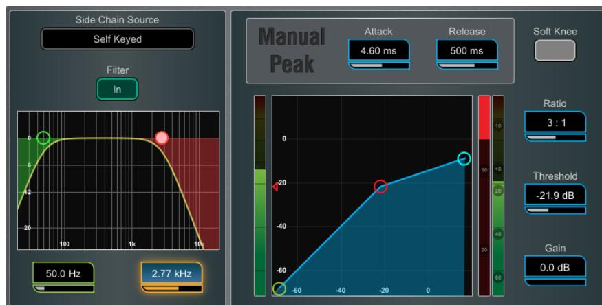
**Manual Peak** - Offers the response of a peak based threshold detector with various smoothing, auto hold/recovery schemes to minimise distortion. The algorithm is capable of ultra fast attack time with minimal lag before onset.
