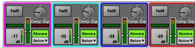
**Comp/Exp** - Sets the maximum amount of compression (EQ cut) or expansion (EQ boost) for the band when the sidechain signal level is 'Above' or 'Below' the threshold setting. Centre position is zero dB flat.
