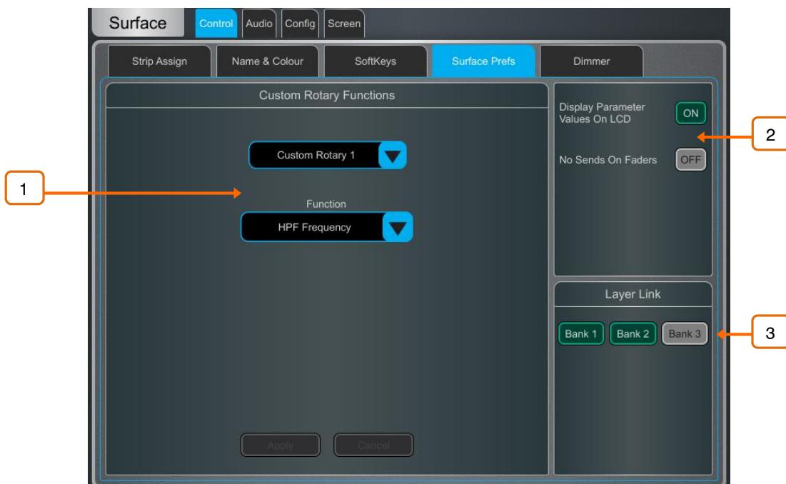
1 **Custom Rotary Functions** – Use the drop-down menus to select the Custom strip rotary control and the required **Function**. Available functions are Unused, Direct Out, Send Level (Aux or FX sends), HPF Frequency, Compressor Threshold, and Channel Level. Touch **Apply** to confirm the change.
