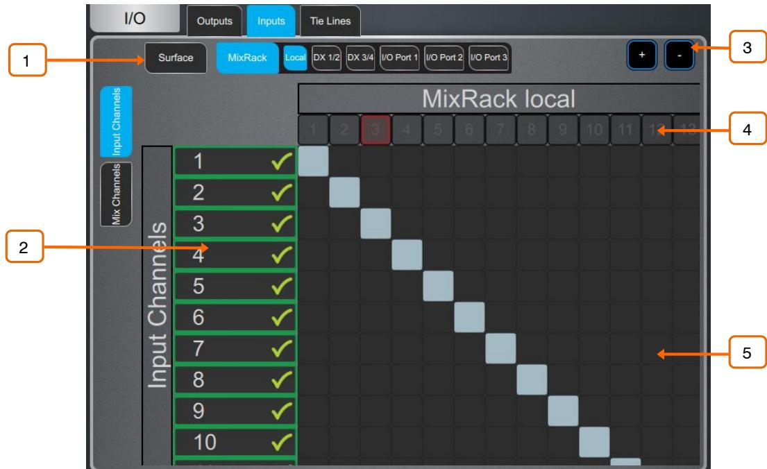
**1 Navigation tabs** – Touch on an item to present its associated sources or channels to the matrix view. Multiple items can be displayed at the same time (**Radio mode** disabled) or one at a time (**Radio mode** enabled).
