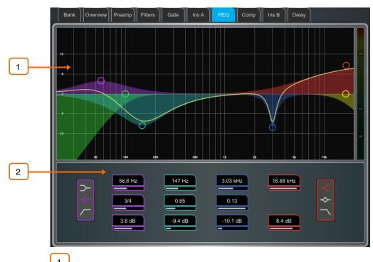
**Graph** – Touch and drag the 4 band dots to adjust their centre frequencies. Touch and drag the HPF / LPF dots to adjust their cut-off frequencies. The overall frequency response curve turns yellow when the PEQ is switched in and grey when switched out.
