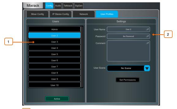
**Users** – The Admin user has access to all functions and can set permissions and allocate passwords if required for the other users. The password, if one is set, is required when the User logs in, changes User or locks / unlocks the dLive Surface. Icons in the list indicate if a password is set and if the User is active.
