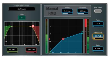
**Manual RMS** - Offers the response of a fairly fast pre-threshold RMS detector with added ability to manually modify the post threshold ballistics for classic sounding RMS compression with additional attack or release smoothing.
