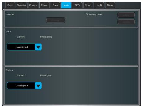
**Insert Unassigned** – Use the drop-down menus to assign the **Send** and **Return** to physical sockets, the I/O Ports or an FX unit. Touch **Apply** to confirm.
