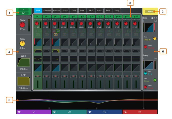
**Selected channel** – Displays the name, colour, type and number of the currently selected channel. Tap to edit channel name and colour. 7 colours and off are available.
