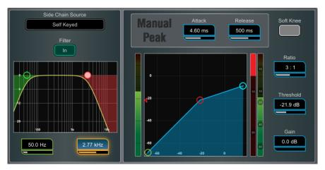
**Manual Peak** - Offers the response of a peak based threshold detector with various smoothing, auto hold/recovery schemes to minimise distortion. The algorithm is capable of ultra fast attack time with minimal lag before onset.
