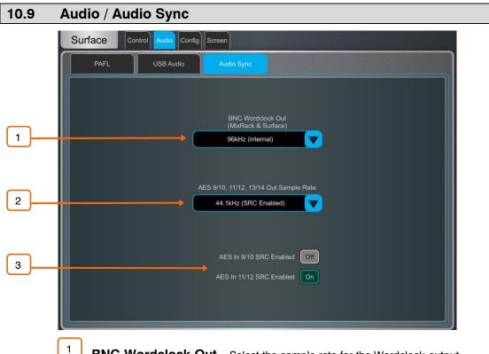
**BNC Wordclock Out** – Select the sample rate for the Wordclock output provided at the Surface and MixRack. This can be set to **Off**, **44.1kHz**, **48kHz** or **96kHz (internal)**.
