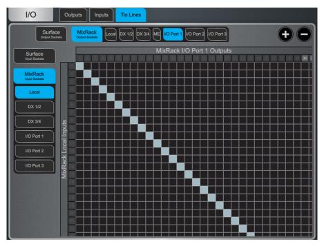
**Digital Split using Tie Lines** – In a digital split system (for example FoH and Monitors), it is typical to use the Tie Lines to send the Local inputs from the Master MixRack to an I/O Port and over to the Slave system, as pictured above. This method (as opposed to using channel Direct Outs) splits the signals straight after the preamp so they are unaffected by Digital Trim or Direct Out Source on the Master system.
