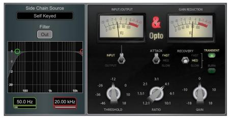
**Opto** - Offers the response of a filament optical compressor. The release has nonlinear exponential recovery, fast at the start and smooth for final recovery stage. This creates a smooth and musical sounding compressor.
