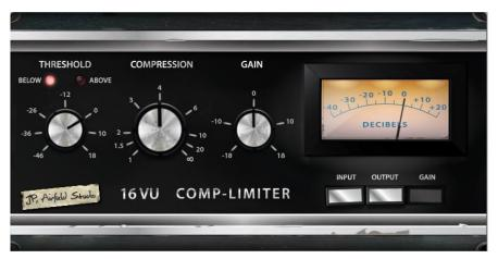
**16VU** - Based on an original vintage VCA based RMS compressor with VU needle meter, with pleasant characteristic sound due to its non-linearity and distortion artefacts, and also with a simple three rotary control interface.
