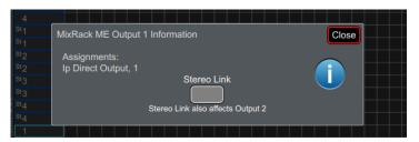
Touch on a ME output to access the Stereo Link option. When Stereo Linked, outputs to the Allen & Heath Personal Monitoring System will be recognised as a stereo pair and assigned to a single key on the ME-1 mixer.
