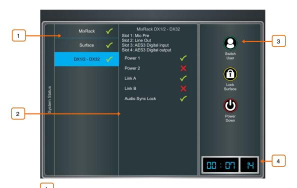
**System Status** – Displays a list of system components. A green tick indicates the component is running correctly. A red cross indicates that an error is detected. Touch the component to display further information.
