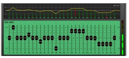
**Digi-Q** - Gain and width are optimised to minimise band interaction and to provide a frequency response as close to the slider positions as possible.
