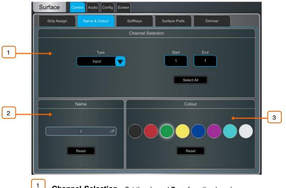
**Channel Selection** - Set the channel **Type** from the drop-down menu. Touch **Select All** or set the **Start** and **End** to select a range of channels.
