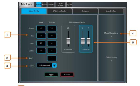
**Bus configuration** – Touch a box and use the screen rotary to set the number of mono / stereo Groups, FX sends, Aux sends and Matrix outputs. You can choose any combination, but note that mono busses can only be added / removed in pairs.
