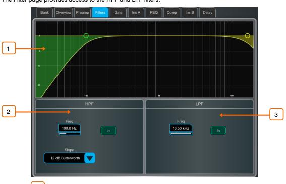
The Filter page provides access to the HPF and LPF filters.
