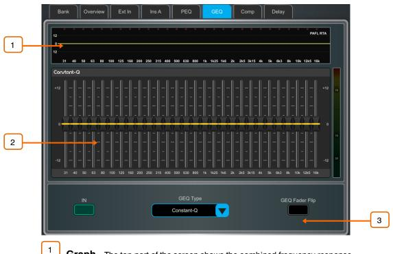
**Graph** – The top part of the screen shows the combined frequency response curve of the GEQ. The curve turns yellow when the GEQ is switched in and grey when
