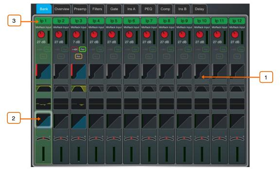
**Input channels** – Displays name and colour, source type, preamp meter, gain, +48V and polarity, gate graph, filters, PEQ graph, compressor graph, Pan and channel meter.
