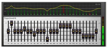
**Proportional-Q** - Provides smooth wide Q for low cut/boost, which progressively tightens beyond 1/3rd octave for max boost/cut.
