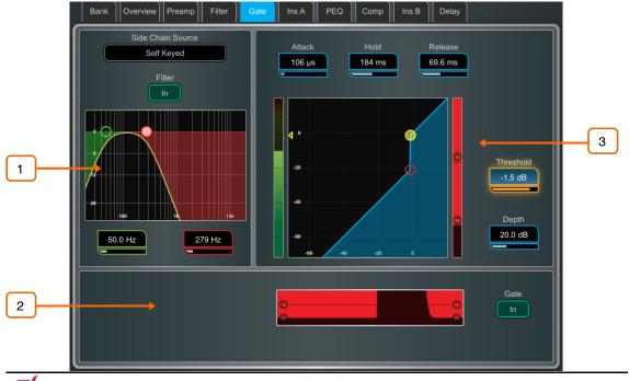
**Side Chain** – Touch the **Side Chain Source** box to open a window for selecting the Key (trigger) input to the Gate. An adjustable HPF and LPF filter can be switched in to limit the frequency range of the Key signal. The curve turns yellow when the filter is switched in.
