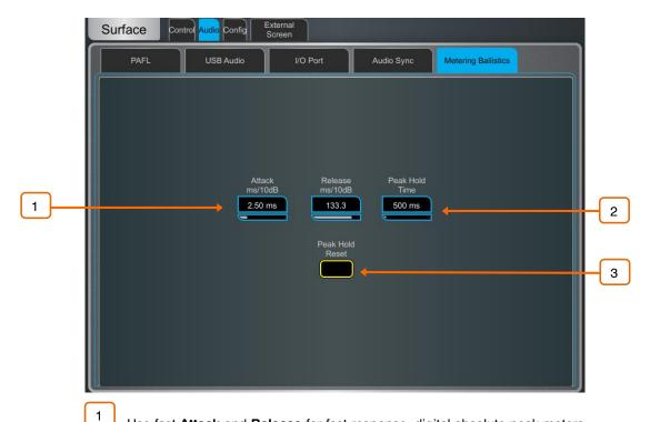
Use fast **Attack** and **Release** for fast response, digital absolute peak meters. This ensures you keep control and avoid digital clipping of signals including those with very fast dynamics, but note that the meters may read hotter than those on other consoles you are used to.
