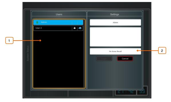
**Users list** - Shows available Users. These can be configured and enabled in the MixRack / Config / User Profiles screen. The Admin User is always displayed. Icons indicate if the User has a password or User Scene set. Touch a User to select then touch Login to change User.
