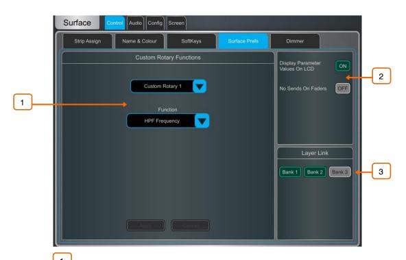
**Custom Rotary Functions** – Use the drop-down menus to select the Custom strip rotary control and the required **Function**. Available functions are Unused, Direct Out, Send Level (Aux or FX sends), HPF Frequency, Compressor Threshold, and Channel Level. Touch **Apply** to confirm the change.
