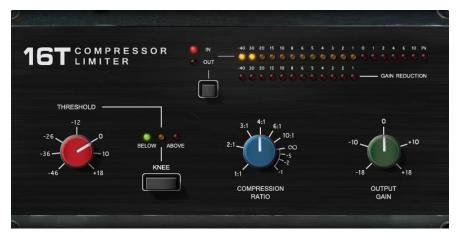
**16T** - Inspired by an industry classic VCA based RMS compressor this model produces a tight, punchy compression particularly useful with live bass and percussion and also vocals, and with a very easy to use three rotary control interface.
