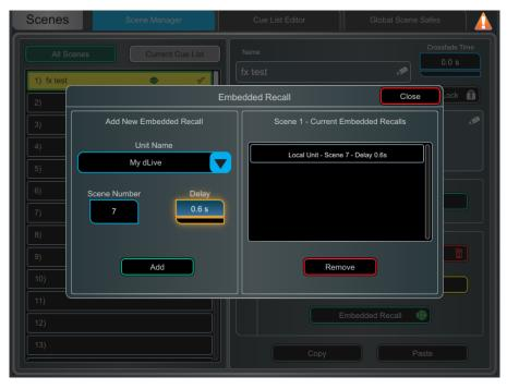
**Embedded Recall** – You can automate the recall of one or more other Scenes from the same or a different unit when you recall a Scene. A delay time can be set for each embedded Scene within the host Scene.
