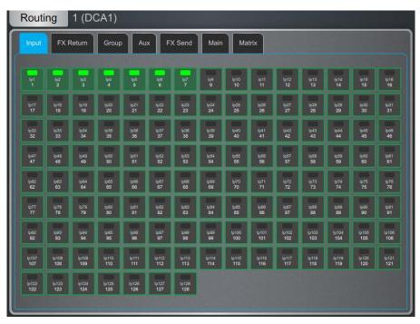
**DCA and Groups** – Displays channel assignments to the DCA or Group. Touch **On/Off** to toggle the channel assignment to the DCA or Group. For DCAs, use the tabs on top to display different channel types.
