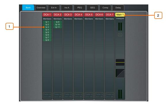
**DCAs** – Displays name, colour, members (assigned channels) and whether the 'Fader to Zero dB' option is enabled. Use the **Routing** screen or the Surface **Assign** keys to assign channels.
