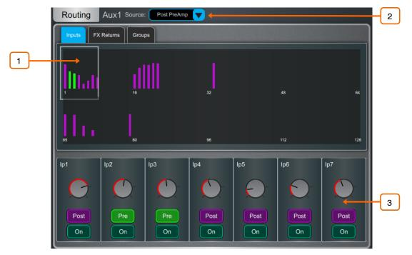
**Aux and FX sends** – Displays routing and assignments of Input channels, FX Returns and Groups to the selected Mix.
