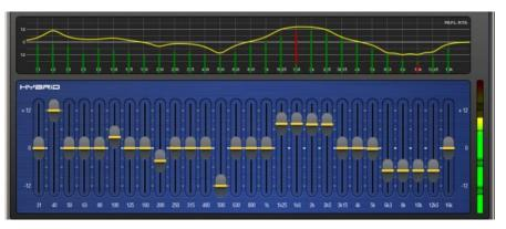
**Hybrid** - Allen & Heath have developed the best of both worlds. The boost is proportional-Q for smooth and warm small boost settings. The cut is Constant-Q providing clinical 1/3rd Octave attenuation with minimal band interaction.
