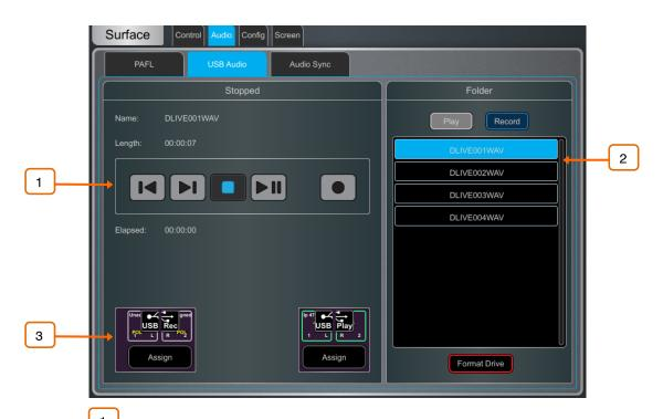
Use the transport buttons to Play, Pause, Stop, Record and select previous or next track. To record, press Record to arm the recording, then press Play.
