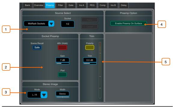
**Source Select** – Open the drop-down menu to choose which source to patch to the channel, touch the **Socket** box then turn the screen Rotary to select the required socket or channel number, then touch **Apply**.
