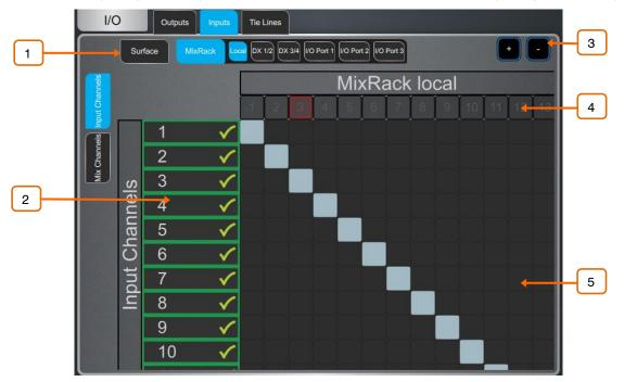
**Navigation tabs** – Touch on an item to present its associated sources or channels to the matrix view. Multiple items can be displayed at the same time (**Radio mode** disabled) or one at a time (**Radio mode** enabled).
