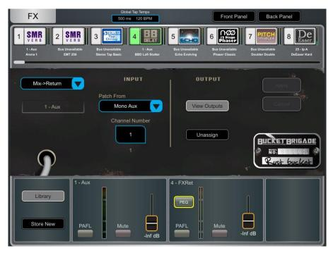
**Back Panel** – Use this view to edit the routing for the selected FX. Use the dropdown box to choose between Unassigned, Insert or Mix->Return.
