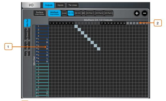
**Sources** – Channel names and colours are displayed. Touch a channel name or number to edit its name and colour.
