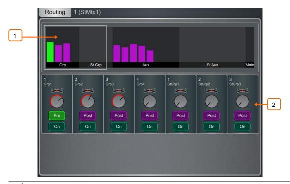
$\ensuremath{\textit{Matrix sends}}$  – Displays routing and assignments of Groups, Aux and Main mixes to the selected Matrix.
