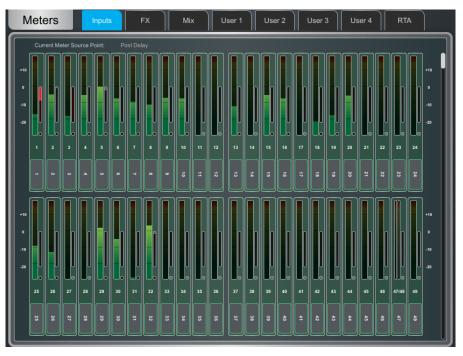
**Meters tabs** – Channel name and colour is shown below each meter. A gain reduction meter and gate active indicator are also displayed, these show activity in red when switched In, and in grey when switched out.
